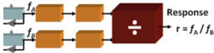
Figure 2-7: Layout of Ring Oscillator with division counter measure and compensation mechanism.
