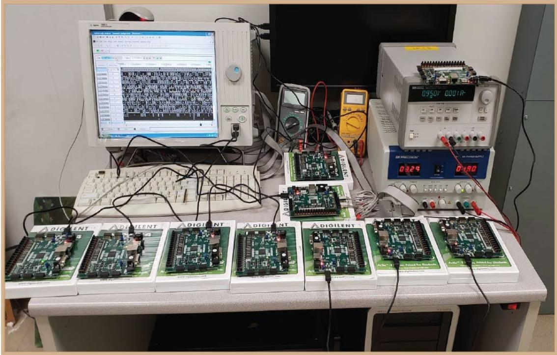
Figure 4-4: Experimental setup for aging with voltage variations experiment.
