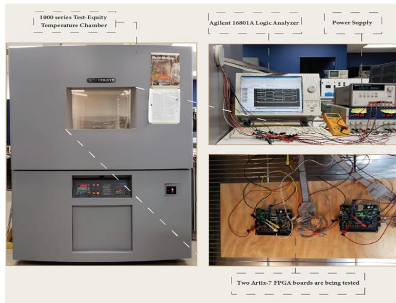
Figure 5-1: Experimental setup for temperature with voltage variations experiment.
