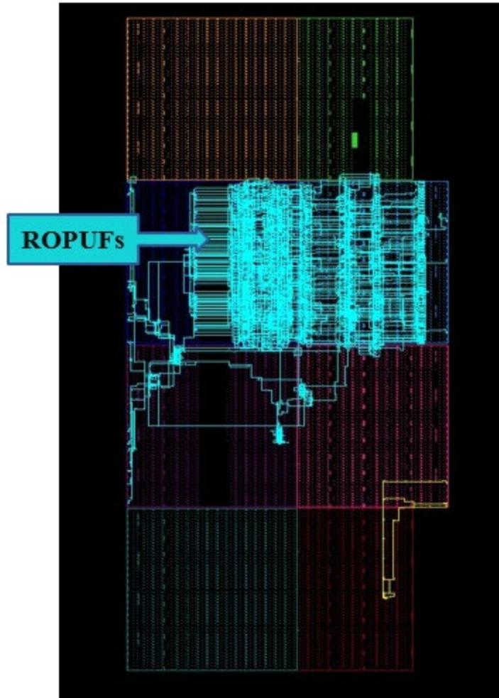
Figure 7-5: 512 Ring Oscillators mapped on an Artix-7 FPGA board.
