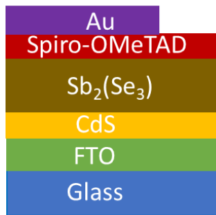
Figure 2- 7: Structure of \text{Sb}_2(\text{S},\text{Se})_3 solar cell in the superstrate configuration.
