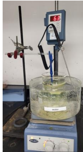
Figure 2- 5: Setup for Cadmium sulfide deposition.
