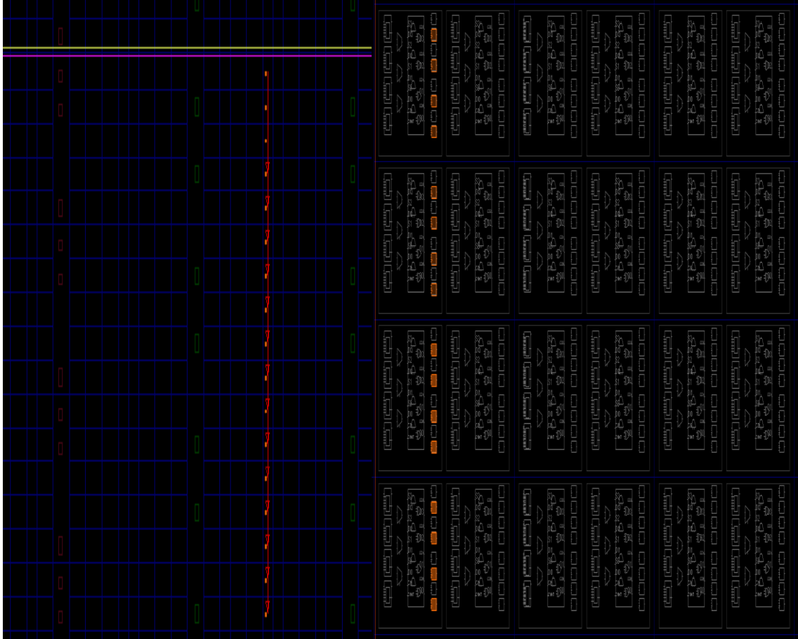
Figure 6-5: Manual Routing of Arbitrator PUF
