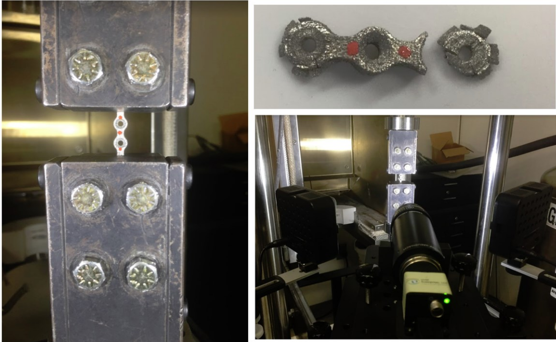
Figure 4-20 Mechanical setup used for the tensile test (Gripper, video extensometer, and a failed sample)
