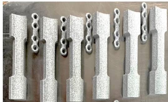
Figure 4-34 NiTi porous bone fixation plates and tensile samples fabricated via the SLM method.
