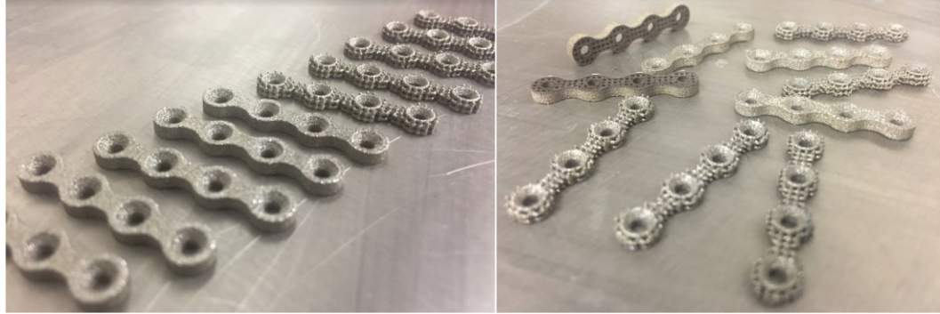
Figure 4-18 Fabricated porous skeletal fixation plates for the mechanical evaluation
