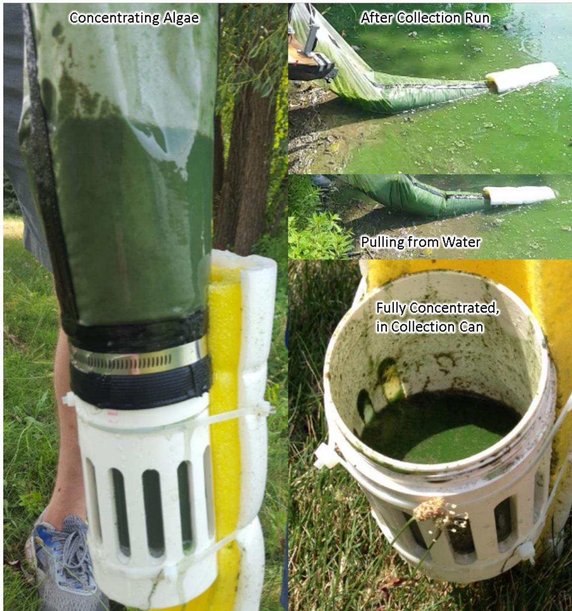
Figure 5-3: Steps in the algae concentration process from immediately after the run (top right), to pulling the boat and net from the water (middle right), to concentrating the algae using agitation (left), until the algae is fully concentrated in the collection can (bottom right).
