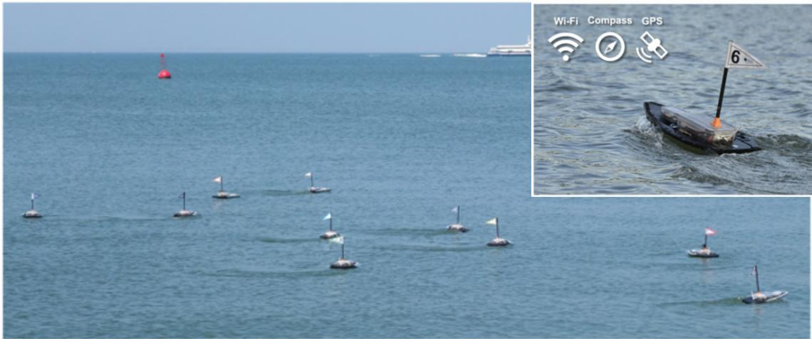
Figure 2-1: Aquatic swarm created by Biomachines Lab at the University of Lisbon, Portugal [32].
