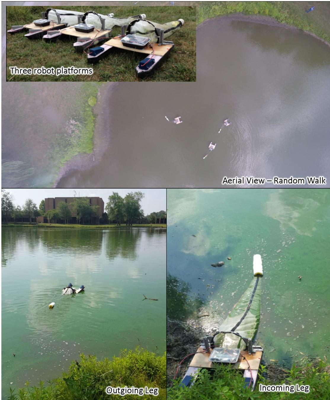
Figure 5-2: (top) Aerial view of three boats performing a random walk further from shore, where the algae is less concentrated. The platforms themselves are visible, as well as the collection can at the trailing end of each net. The inset image shows the three boats side by side. (bottom) Single-boat trial in the much denser algae near the shore showing the (left) outbound and (right) inbound legs of the collection run.
