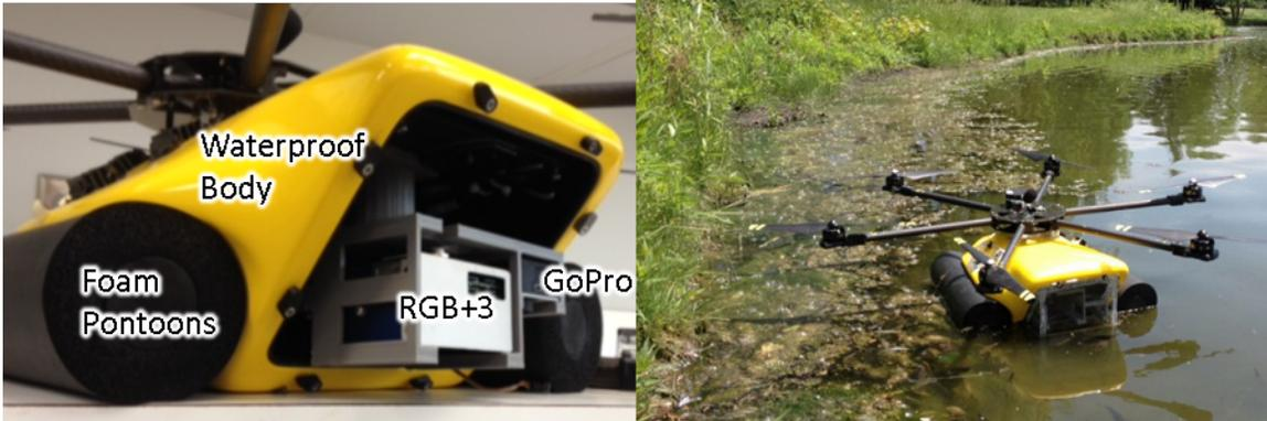
Figure 5-6: (Left) Hexacopter body with Tetracam RGB+3 and Go Pro mounted in a custom bracket, and (Right) Hexacopter landing on the water.
