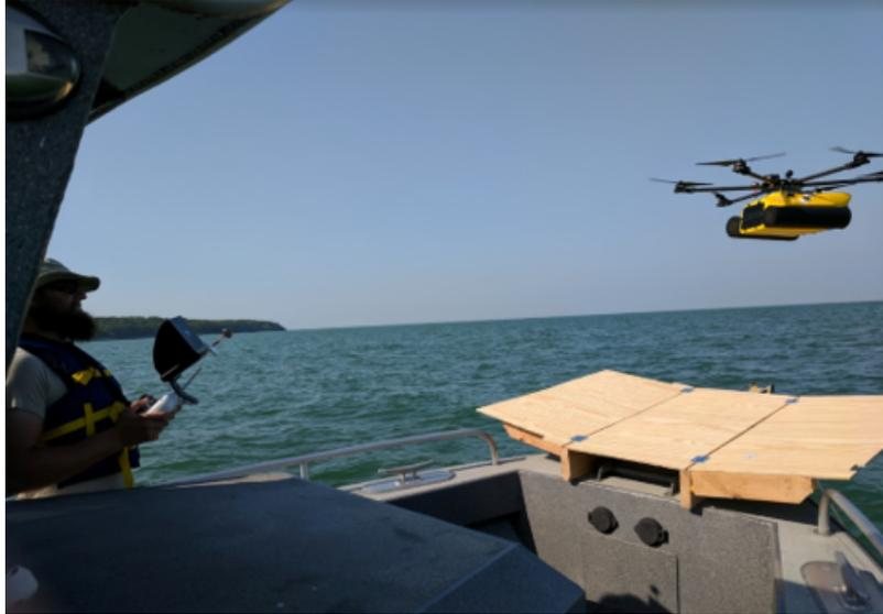
Figure 5-7: Flights from the LEC boat were launched and recovered using a deployable flight deck.
