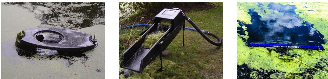
Figure 2-7: (left) propondandlakes.com’s Proskim system’s in-water floating collection unit; (center) Proskim system’s onshore filtration unit; (right) weedersdigest.com’s hand-cast parachute skimmer
