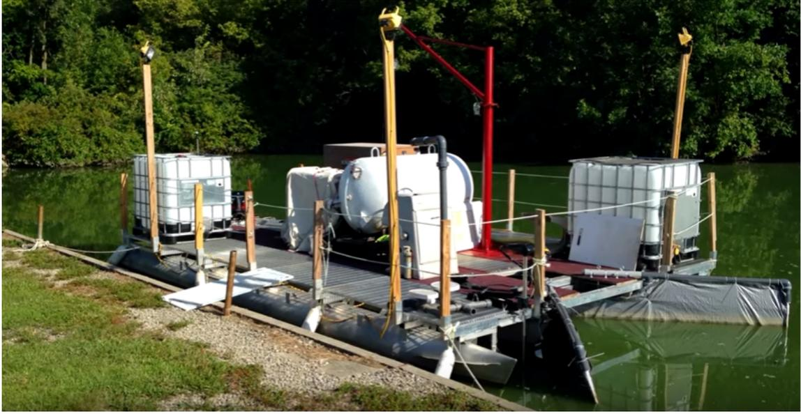
Figure 2-6: Dissolved air flotation system mounted on a mobile platform, taken from Mr. Bryan's submission video for the 2016 Barley Prize
