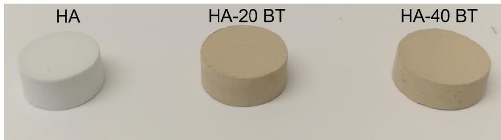
Figure 3-1: HA-x BT sintered samples at 1200°C for 1h
