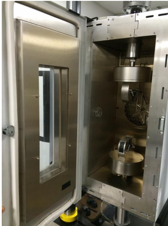
Figure 3-6: Instron 3119-506 environmental chamber attached to the Instron 8801 testing machine.
