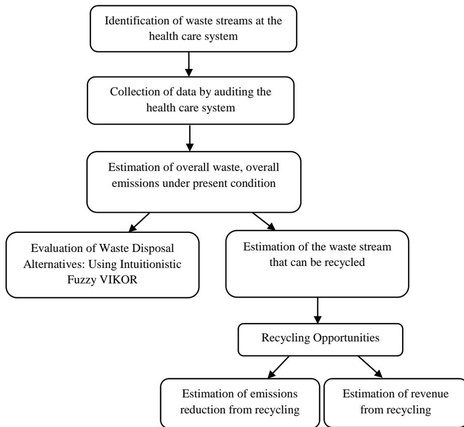
Figure 5-1: Flow chart of generalized model to evaluate waste disposal alternatives, recycling opportunities, GHG emission, and revenue from recycling program
