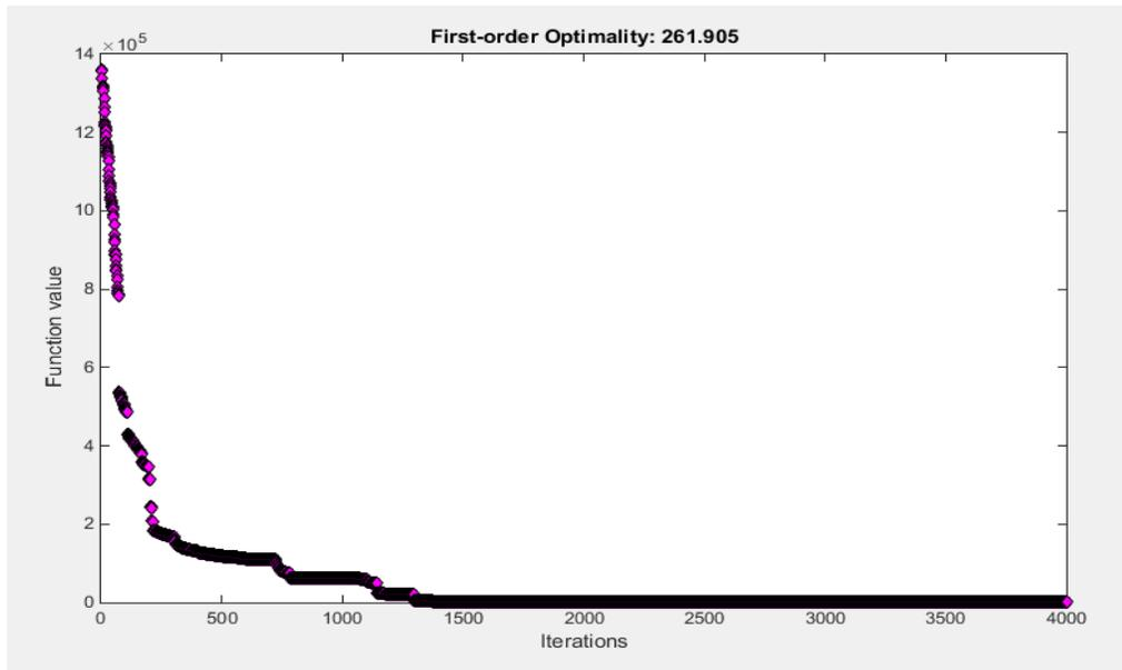
Figure 3-25: Achieved first-order optimality for the best solution found by FminCon (minimum service level 0.7, maximum service level 1, Random set#3)
