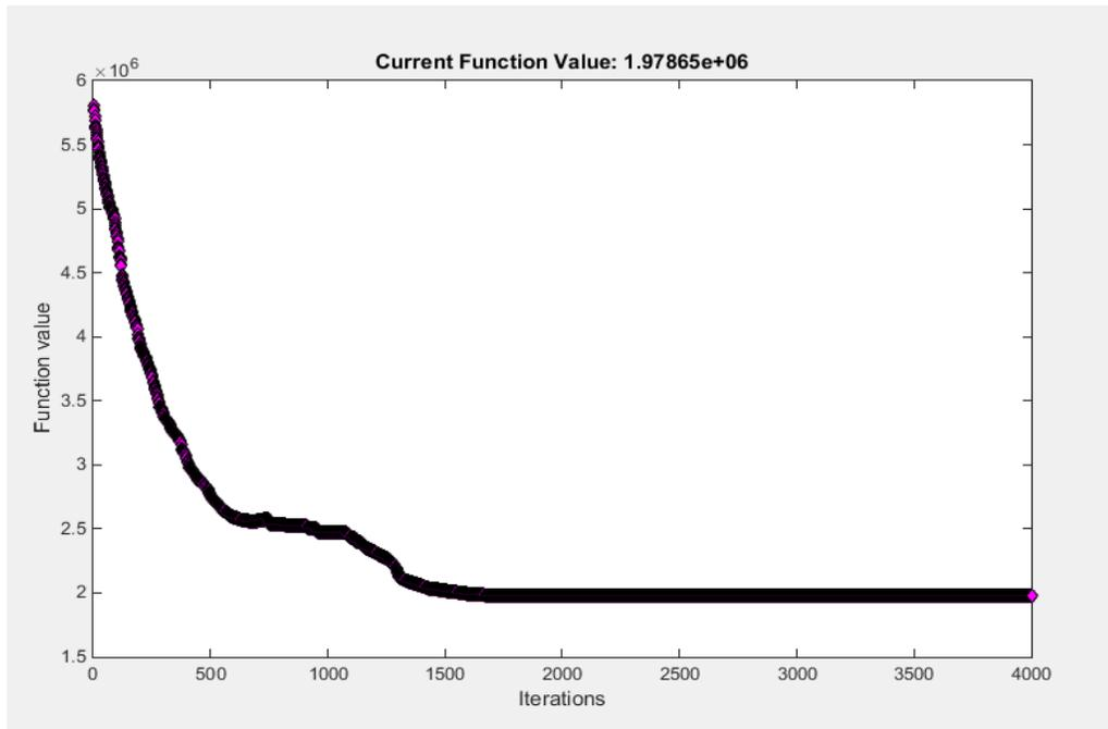
Figure 3-27: Achieved current function value for the best solution found by FminCon (minimum service level 0.7, maximum service level 1, Random set#4)
