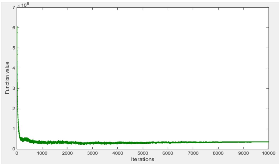
Figure 3-56: Achieved current function value for the best solution found by Grey Wolf Optimizer algorithm (minimum service level 1, maximum service level 1, Random set#4)
