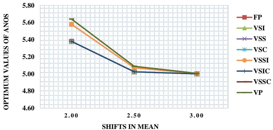
Figure 4-10: The optimum values of ANOS for various ranges (small, medium, and relatively large) of shifts in mean with respect to seven adaptive control charts and the FP chart
