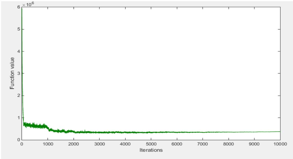
Figure 3-55: Achieved current function value for the best solution found by Grey Wolf Optimizer algorithm (minimum service level 1, maximum service level 1, Random set#3)
