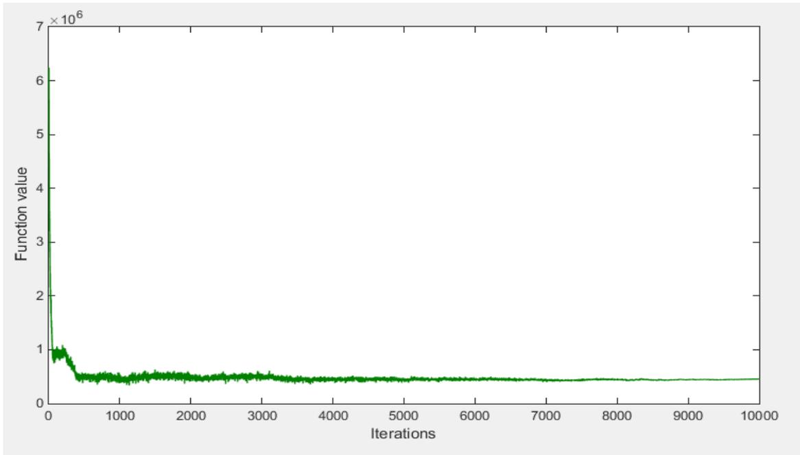
Figure 3-54: Achieved current function value for the best solution found by Grey Wolf Optimizer algorithm (minimum service level 1, maximum service level 1, Random set#2)
