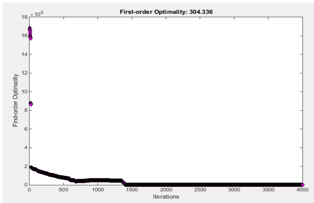
Figure 3-28: Achieved first-order optimality for the best solution found by FminCon (minimum service level 0.7, maximum service level 1, Random set#4)
