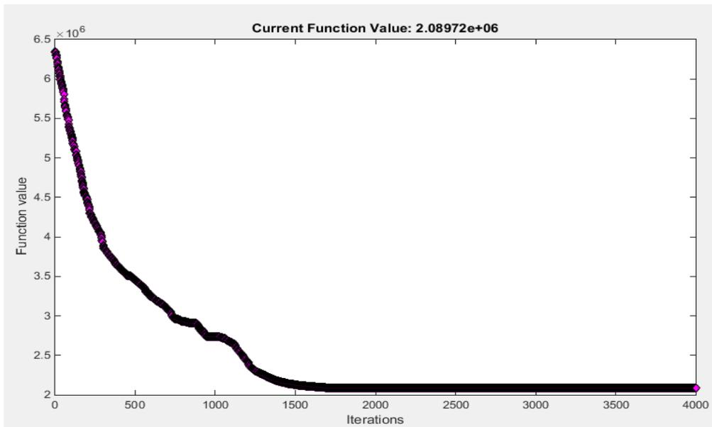
Figure 3-30: Achieved current function value for the best solution found by FminCon (minimum service level 0.7, maximum service level 1, Random set#5)
