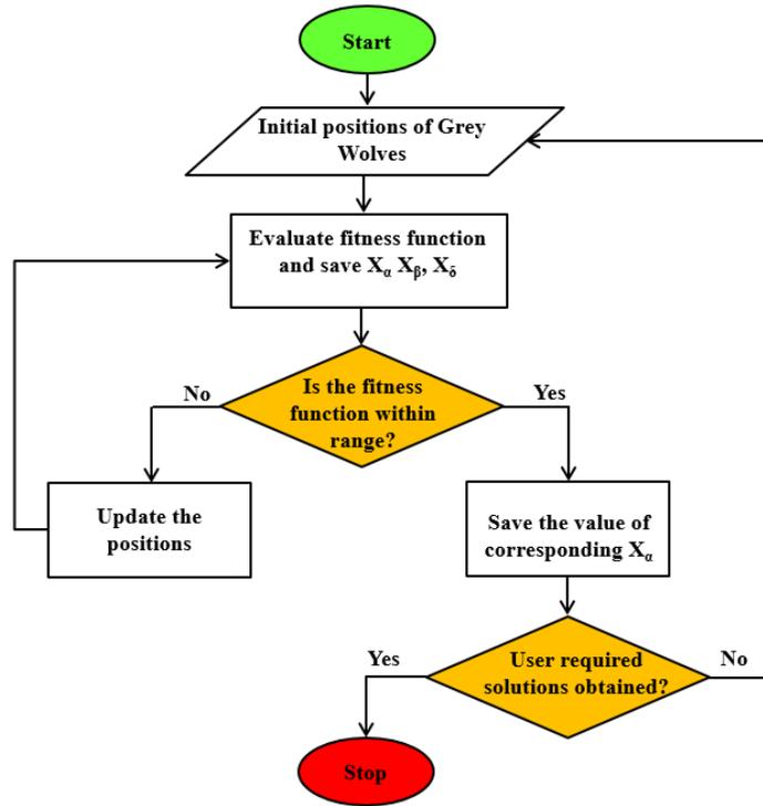
Figure 3-8: The flowchart of Grey Wolf Optimizer algorithm
