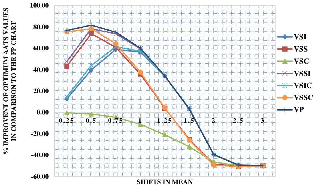
Figure 4-12: The improvement percentages of optimum AATS values for the seven adaptive models in comparison to the FP control chart
