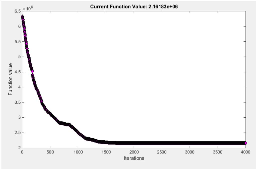
Figure 3-21: Achieved current function value for the best solution found by FminCon (minimum service level 0.7, maximum service level 1, Random set#2)
