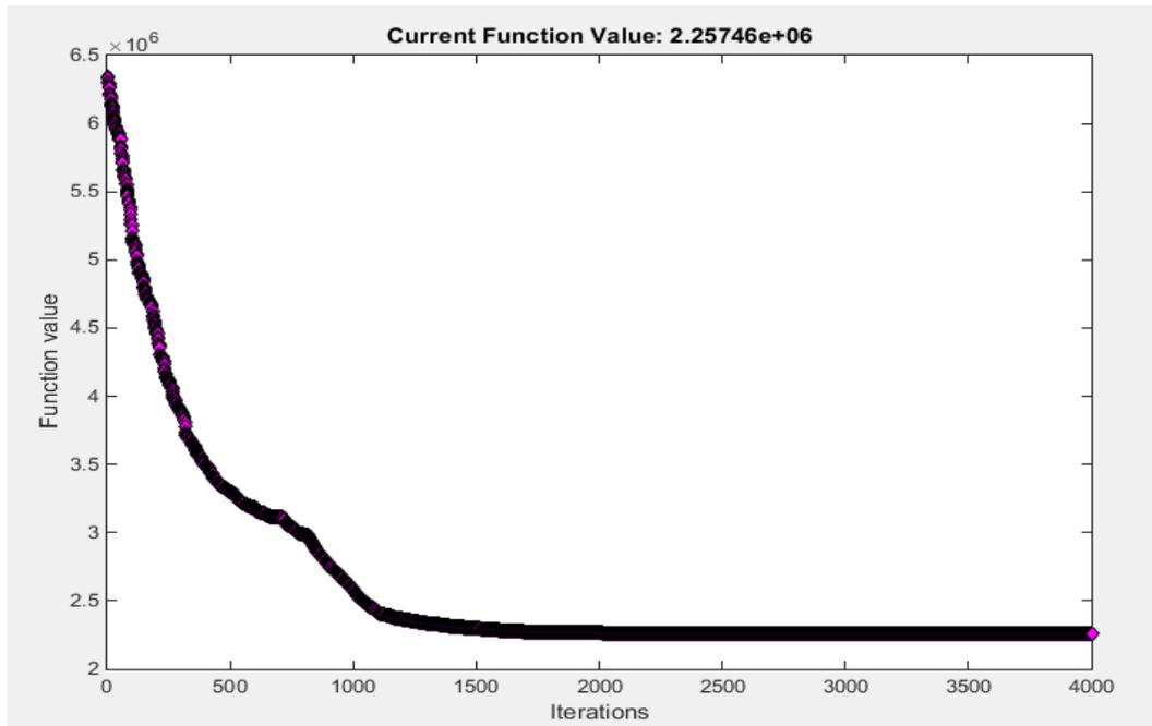
Figure 3-45: Achieved current function value for the best solution found by FminCon (minimum service level 1, maximum service level 1, Random set#5)
