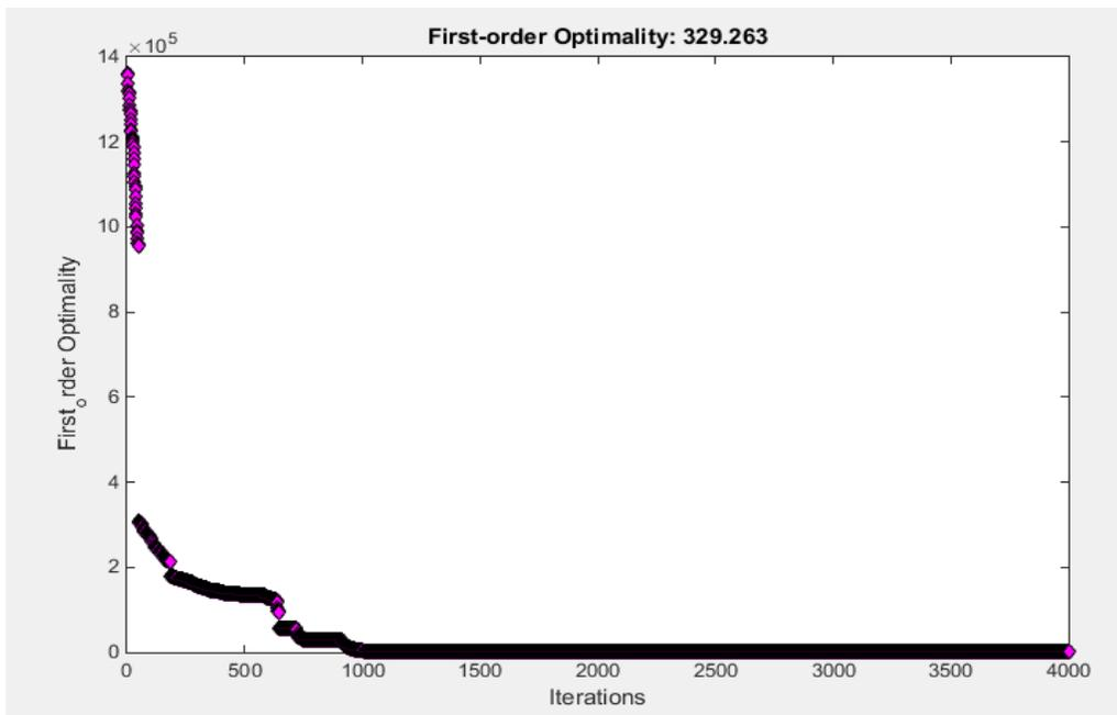
Figure 3-40: Achieved first-order optimality for the best solution found by FminCon (minimum service level 1, maximum service level 1, Random set#3)
