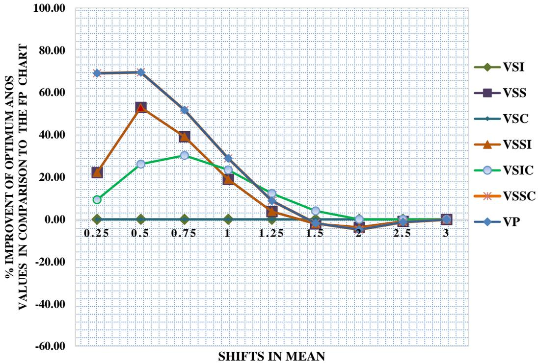
Figure 4-13: The improvement percentages of optimum ANOS values for the seven adaptive models in comparison to the FP control chart
