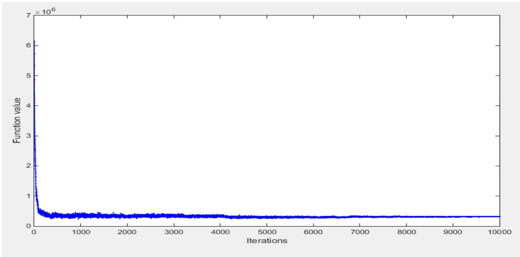
Figure 3-51: Achieved current function value for the best solution found by Grey Wolf Optimizer algorithm (minimum service level 0.7, maximum service level 1, Random set#4)
