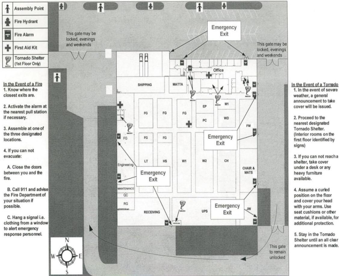
Figure 3-9: Fire and tornado safety plan of an assembler in the considered supply chain network
