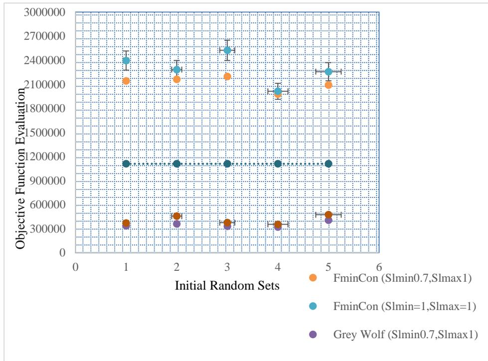
Figure 3-14: Comparing the achieved results for the objective function value by FminCon solver, Grey Wolf algorithm, and Lingo Branch and Bound algorithm
