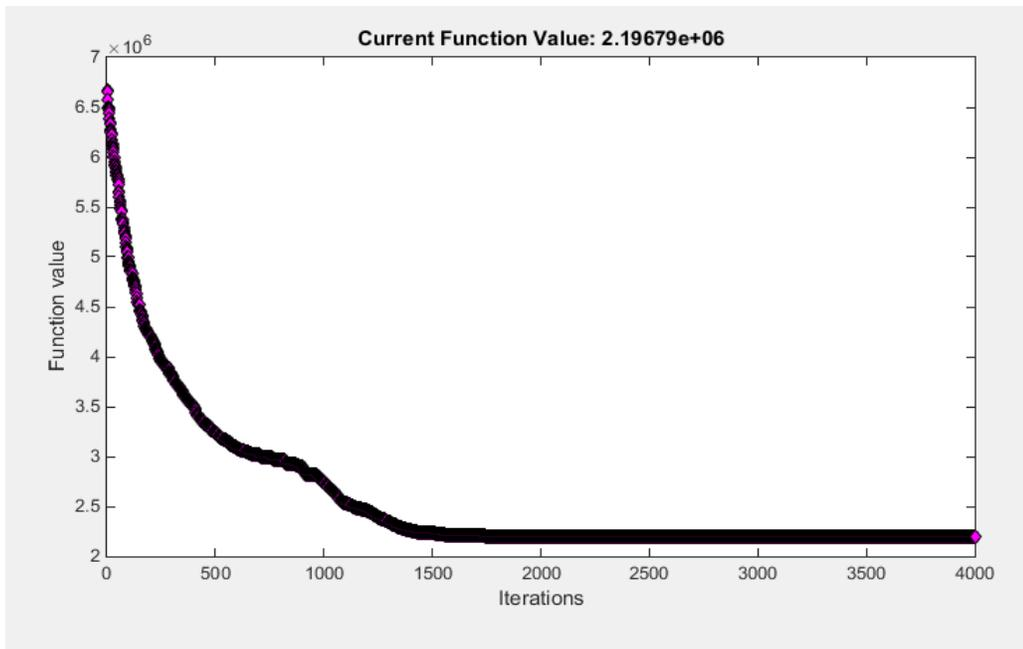
Figure 3-24: Achieved current function value for the best solution found by FminCon (minimum service level 0.7, maximum service level 1, Random set#3)
