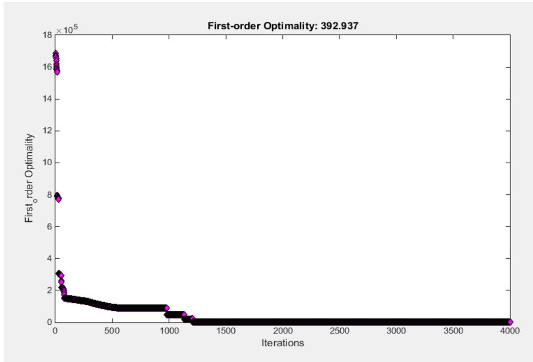
Figure 3-43: Achieved first-order optimality for the best solution found by FminCon (minimum service level 1, maximum service level 1, Random set#4)
