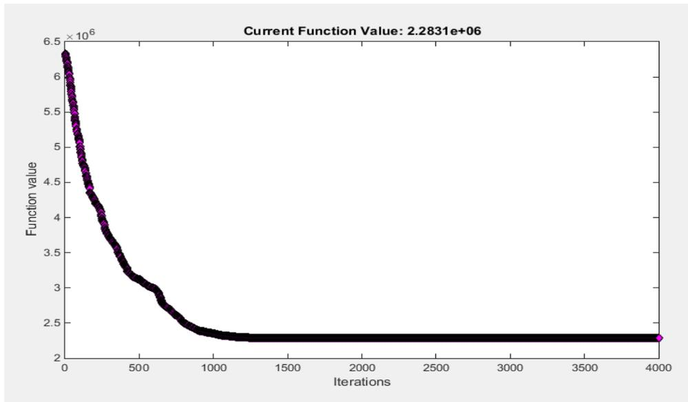
Figure 3-36: Achieved current function value for the best solution found by FminCon (minimum service level 1, maximum service level 1, Random set#2)
