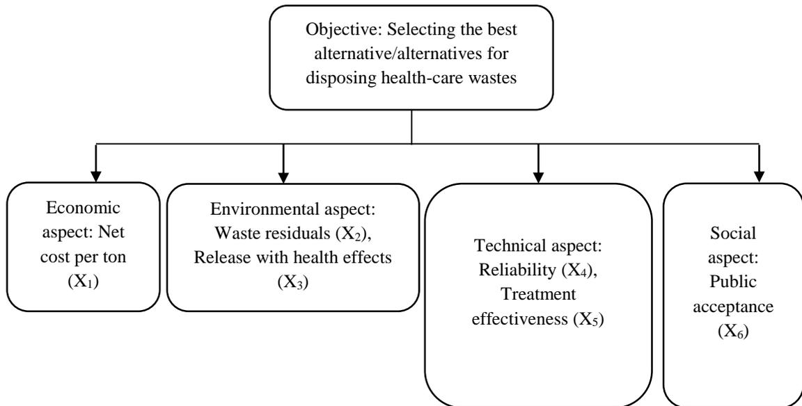
Figure 5-5: Defined criteria and their related sub-criteria for selecting the best alternative/alternatives for health care waste disposal
