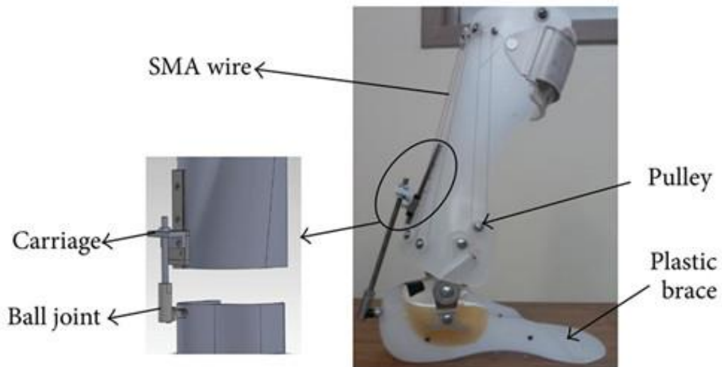
Figure 1-13. The Active Ankle-Foot Orthosis Actuated by Nitinol Wires with Superelastic Effect. The Figure Is Adopted from Reference [37].
