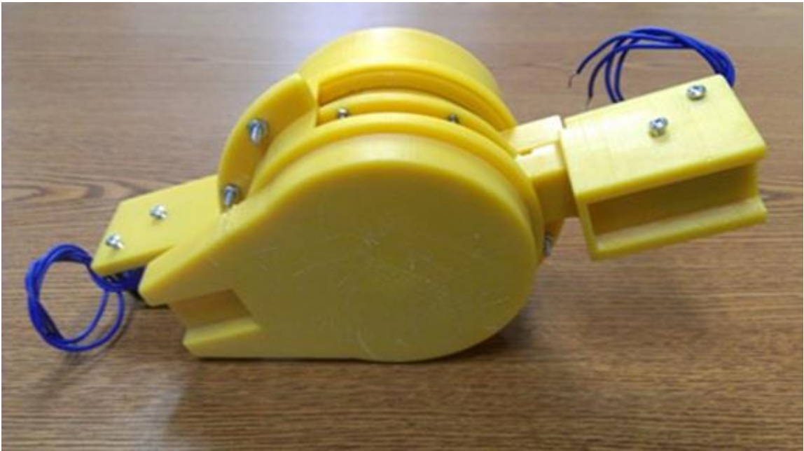
Figure 4-18. The Preliminary Prototype of the Dynamic Knee Module.
