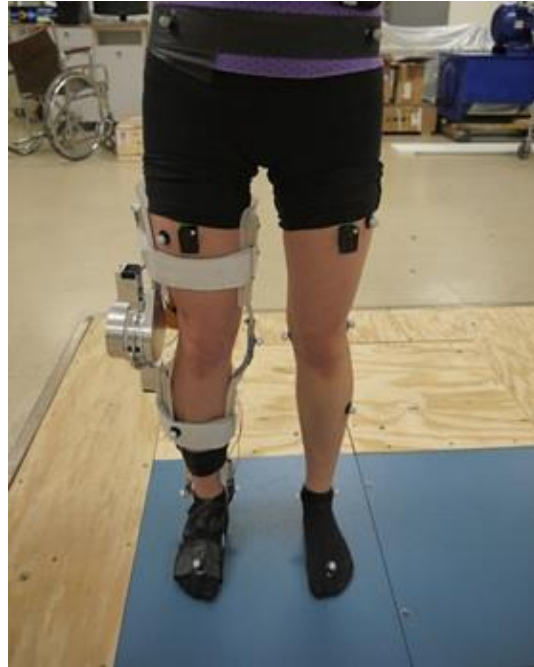
Figure 5-3. The Marker Setup and EMG Sensors When Testing with the UT Dynamic KAFO.
