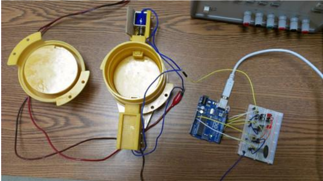
Figure 4-19. The Connection between the Dynamic Knee Module and the Microcontroller.
