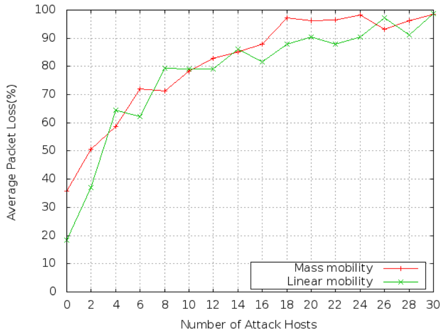
Figure 4-2: Average packet loss for DDoS attack using linear and mass mobility models
