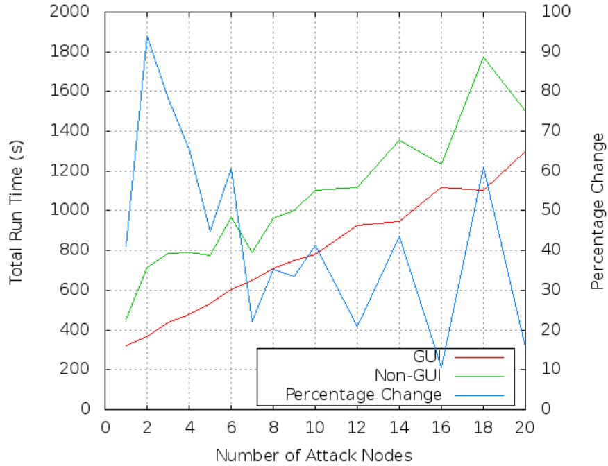
Figure 5-3: Run time variation with GUI and Non-GUI options, and the percentage change in two options for DDoS Attack
