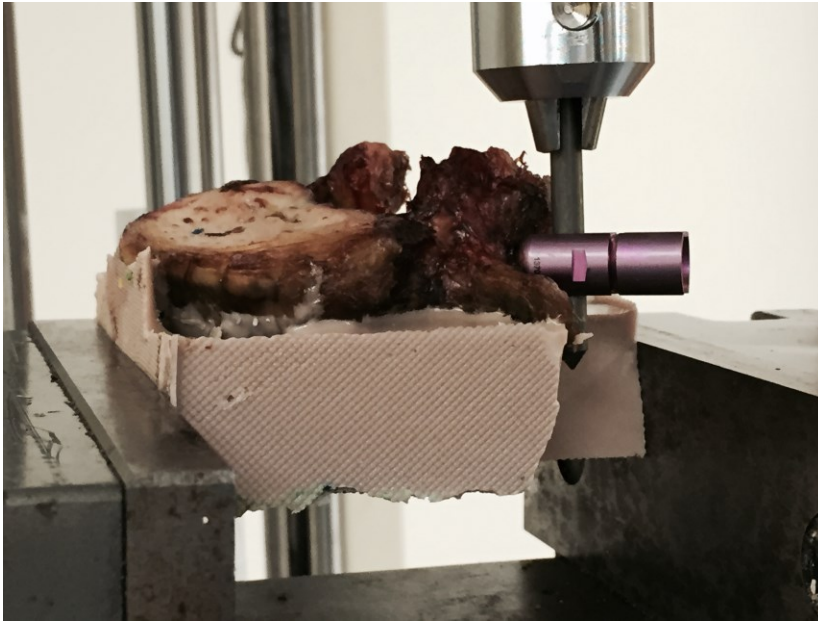
Figure 4-17: The actuator applied the load along the rod to simulate the fatigue.
