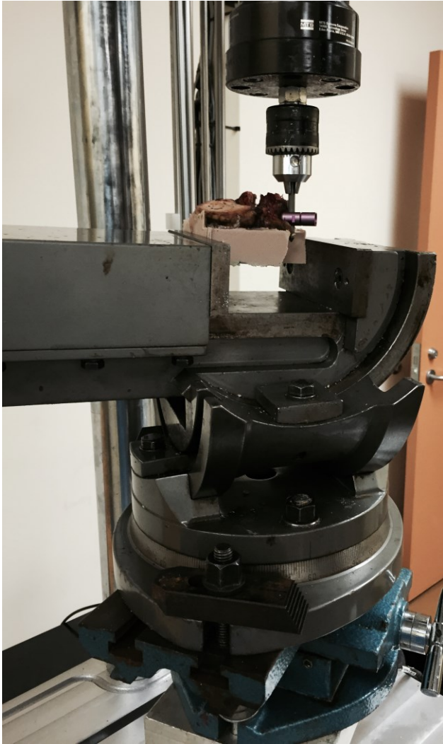
Figure 4-18: The in-vitro setup: 3-axes vice was mounted on top of x-y table top axes to establish proper orientation between rod and actuator.
