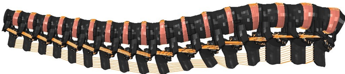
Figure 4-1: FE model of a normal juvenile spine after scaling and adjustment of vertebral body to intervertebral body heights.
