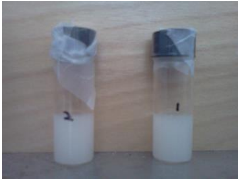
Figure 4-1: Dispersion of AMP in (a) PLA and (b) PLA-HSA system after 24 hours
