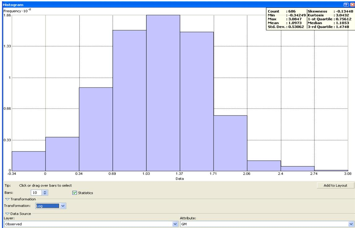
**Figure 4-2: Frequency distribution of the radon dataset after log transformation**
