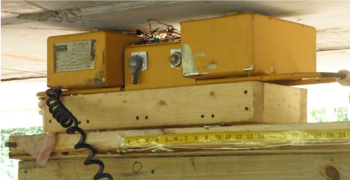
**Figure 4-3: IMF sensing equipment, electromagnet with hall sensors on pole face.**
