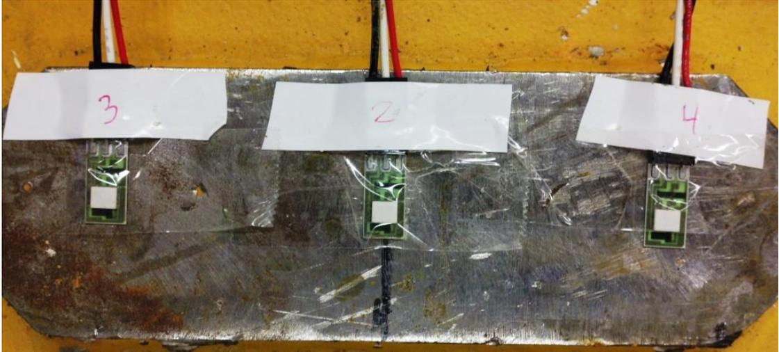
**Figure 3-4: Right pole face sensor layout. Note: Sensor 1 is in same position as Sensor 2 but on the opposite pole face.**
