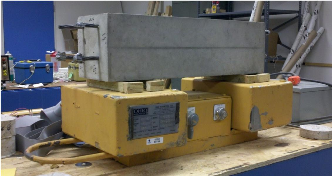
**Figure 3-1: Small scale concrete beam (3/8" Strand).**
