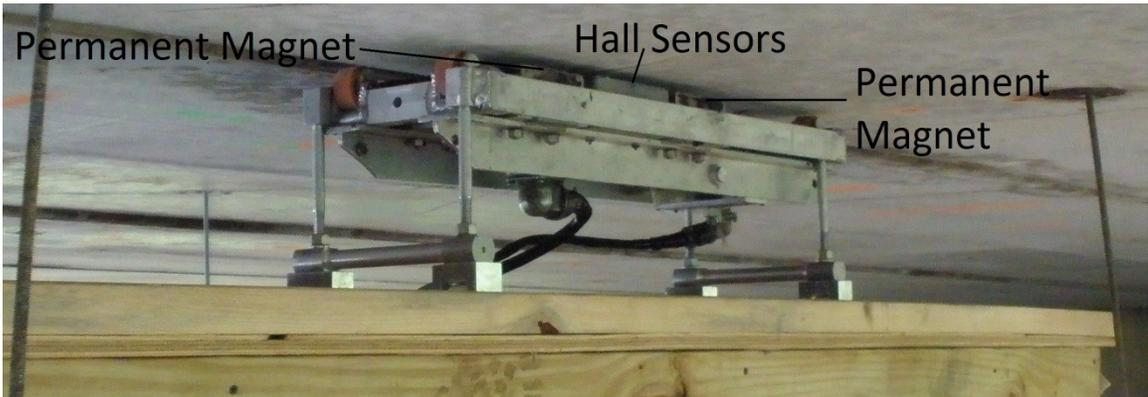
**Figure 4-4: MFL sensing equipment.**
