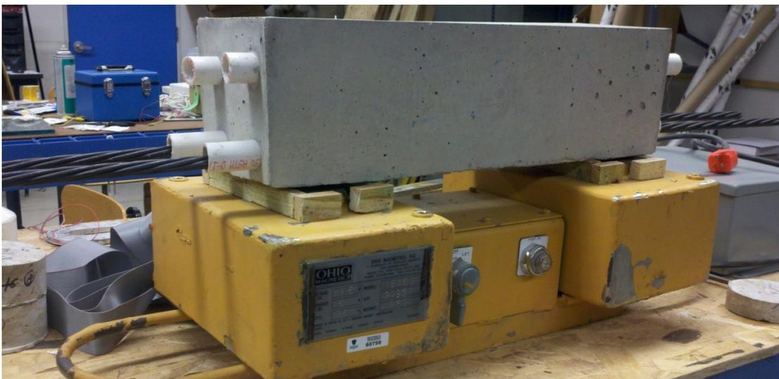
**Figure 3-2: Small scale concrete beam (PVC sleeves).**
