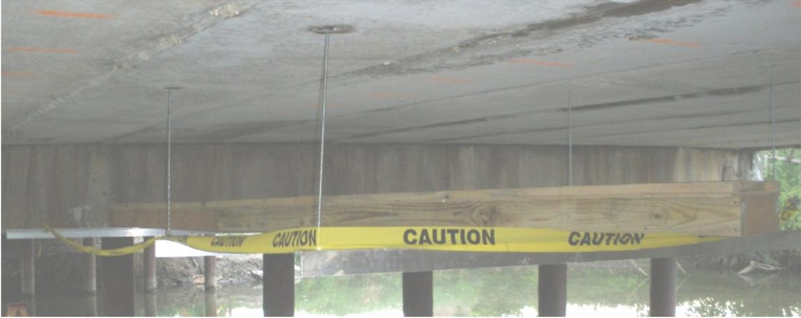
**Figure 4-2: Testing platform attached to bottom of bridge.**
