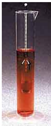
Figure 3-4: A photograph of a Type 152H Hydrometer within a sedimentation cylinder.
