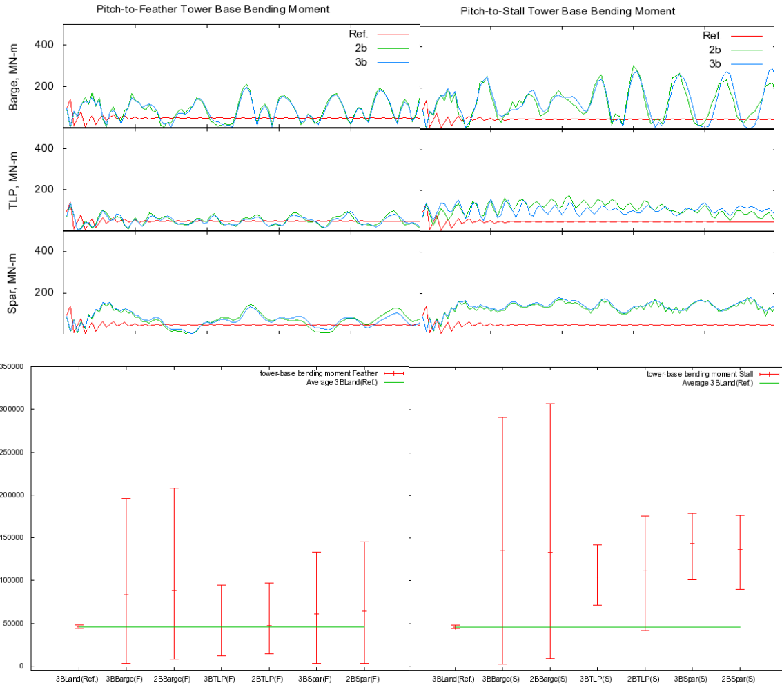
Figure 4.8 – Tower-Base Bending Moment Pitch-to-Feather and –Stall, Time Series and Maximum, Minimum, and Average (See Appendix for larger graphs)
