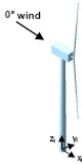
Figure 2.7- tower-base coordinate system [21]
