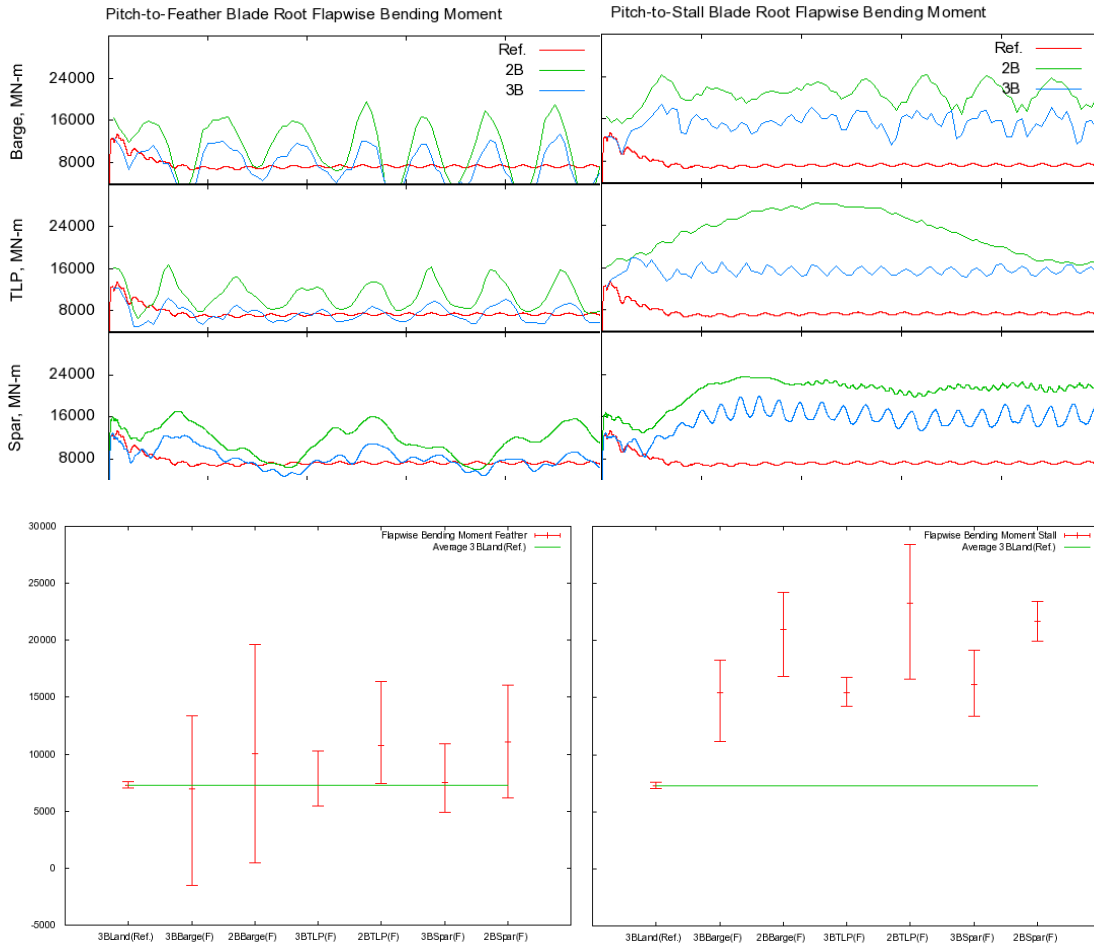
Figure 4.4-4.7 – Blade Root Flapwise Bending Moment Pitch-to-Feather and –Stall, Time Series and Maximum, Minimum, and Average (See Appendix for larger graphs)
