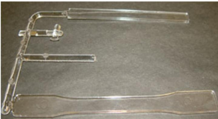
**Figure 2.2.1A** – Photograph of molded part, fatigue test bar on top, tensile test bar on bottom
