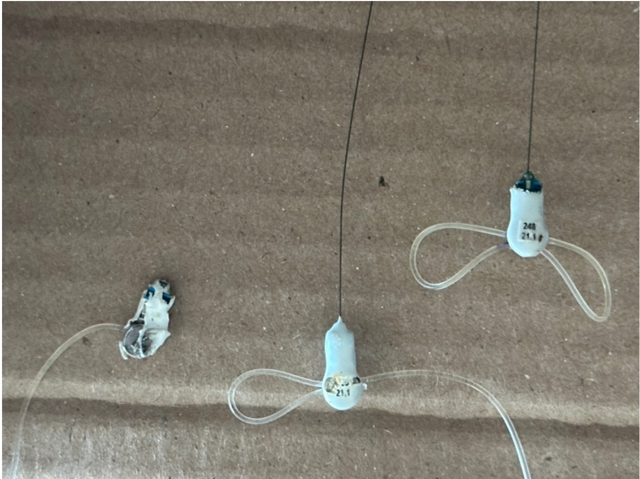
Figure 3.1. Three examples of nanotags damaged by Henslow's Sparrows. Damage was observed to the battery casing, the leg-loop harness, and the antenna.
