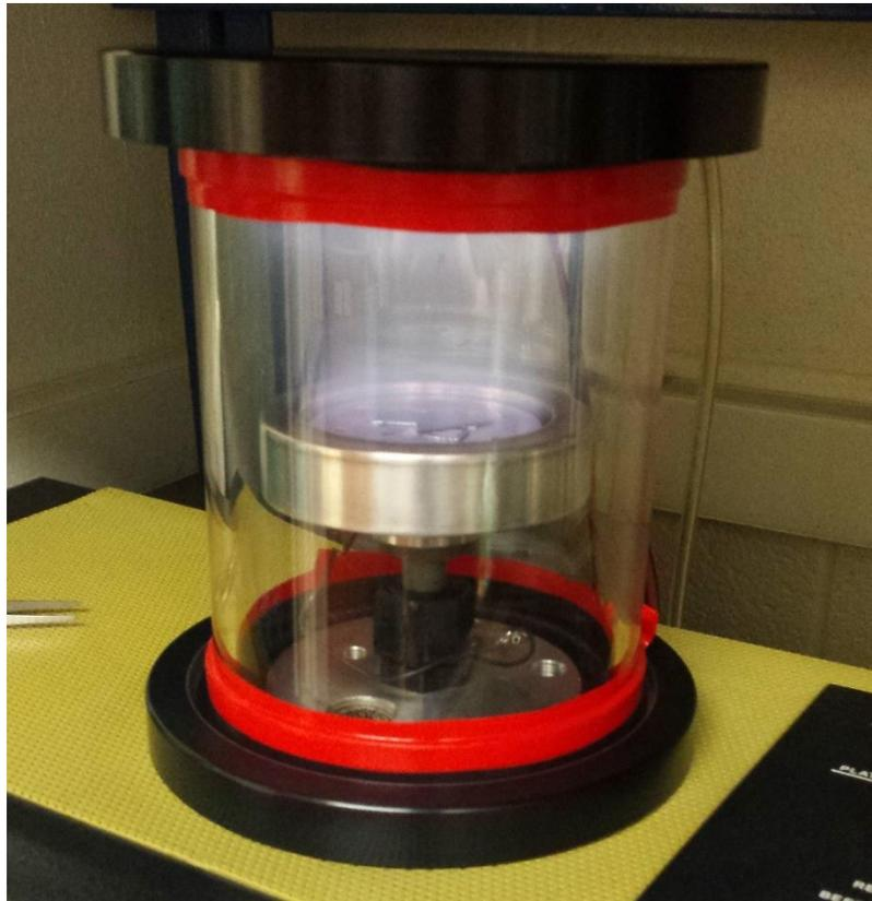
Figure 1.11: A sputtering chamber filled with an oxygen plasma (the light purple glow is the plasma). This chamber is being used to plasma-clean a sample, but was originally designed to sputter.
