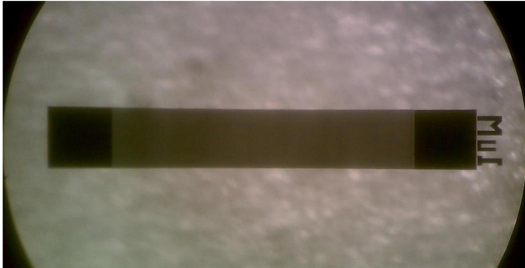
Figure 1.5: One set of interdigitated 1- $\mu\text{m}$  fingers. The fingers lie between two pads, effectively isolating the pads from each other and creating electrodes.
