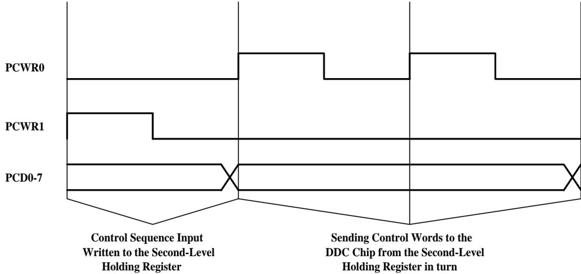
Figure 3.7: Timing Diagram for Loading the Control Words into the DDC Chip
