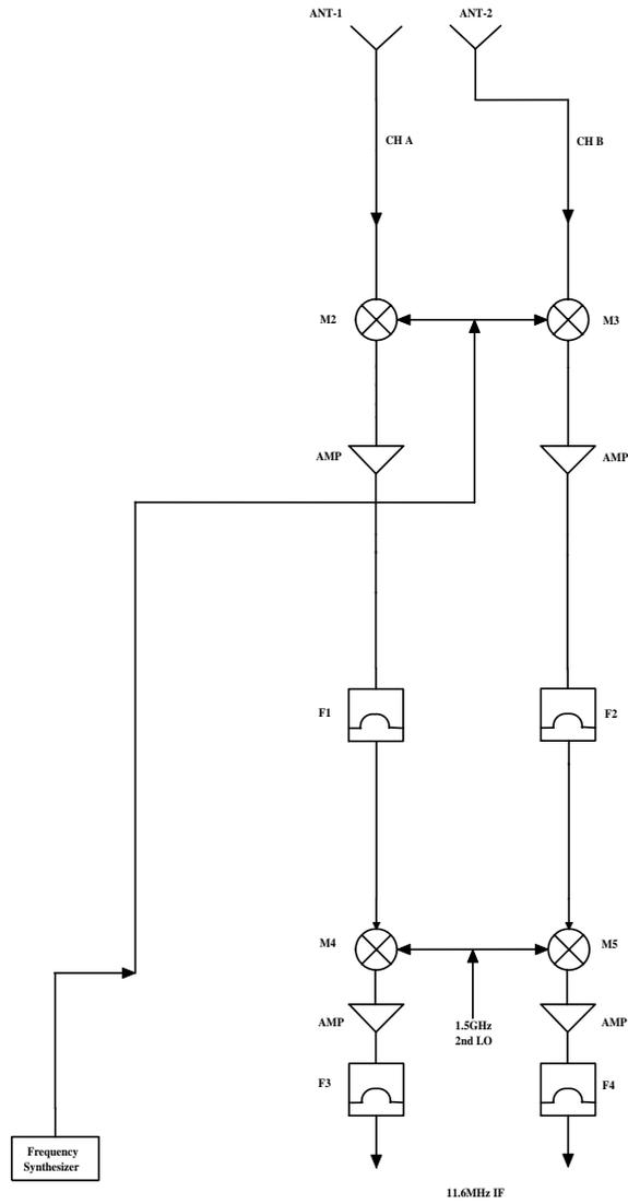
Figure 2.6: The Radar System Diagram of the RF Section (Simplified)
