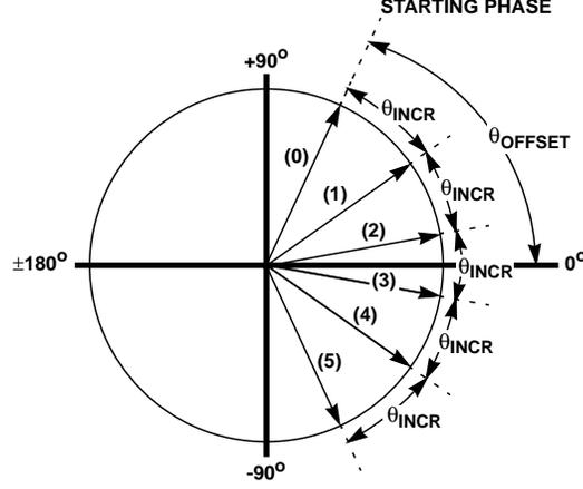
Figure 4.1: Phase Word Parameters for the CW Case
