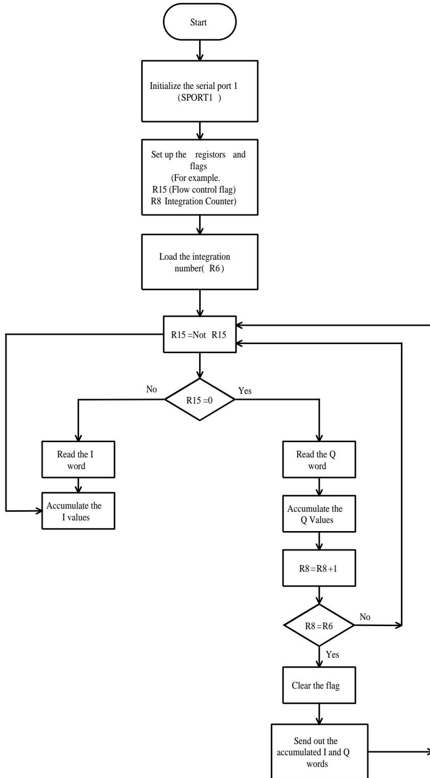
Figure 4.6: Flow Diagram of the DSP Assembly Routine
