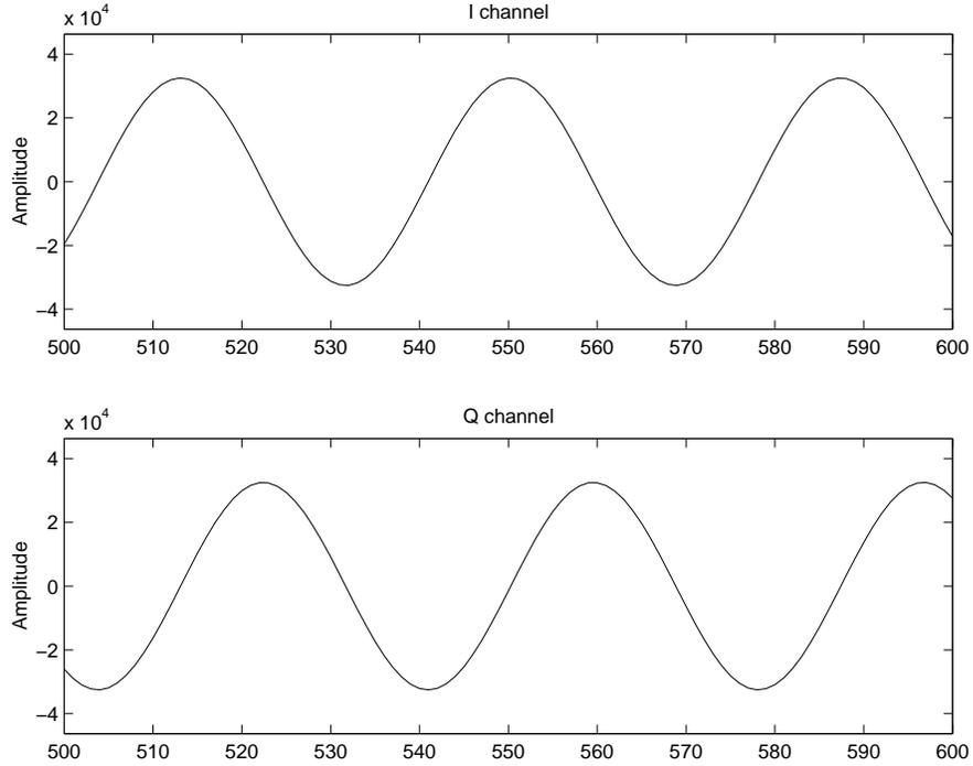
Figure 5.5: Waveform of the I and Q Channel after Downconversion
