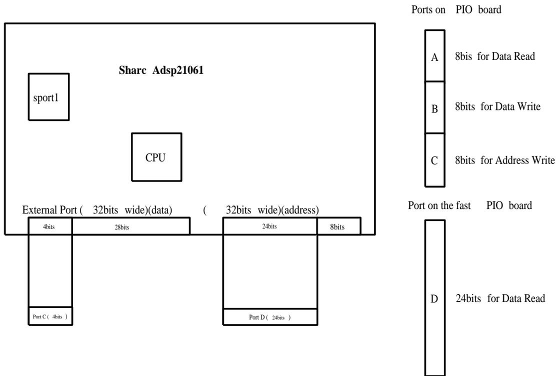
Figure 4.5: The DSP Port Diagram
