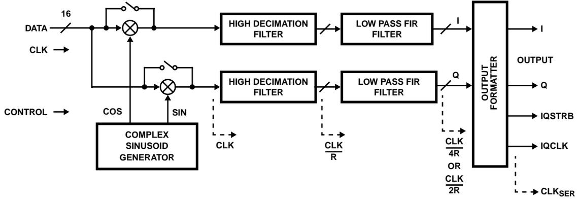
Figure 3.8: Digital Downconverter Functional Diagram
