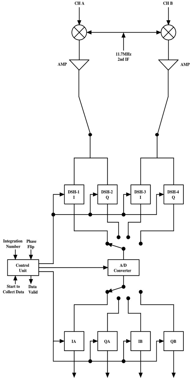
Figure 2.7: The Radar System of the IF Section (Simplified)
