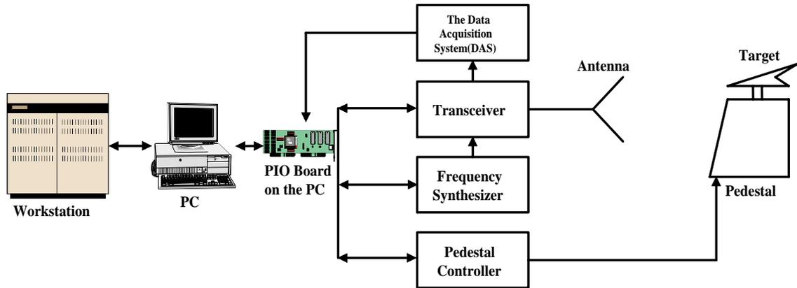
Figure 2.5: The Radar System Diagram
