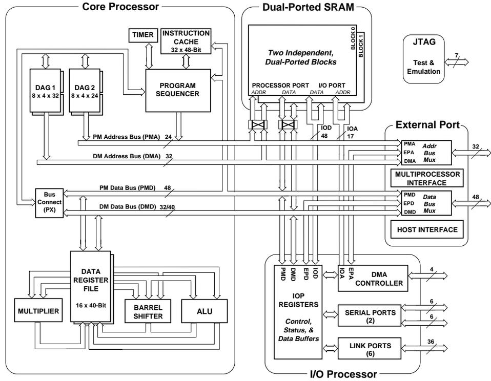
Figure 3.11: ADSP-21061 Data and Address Bus Block Diagram
