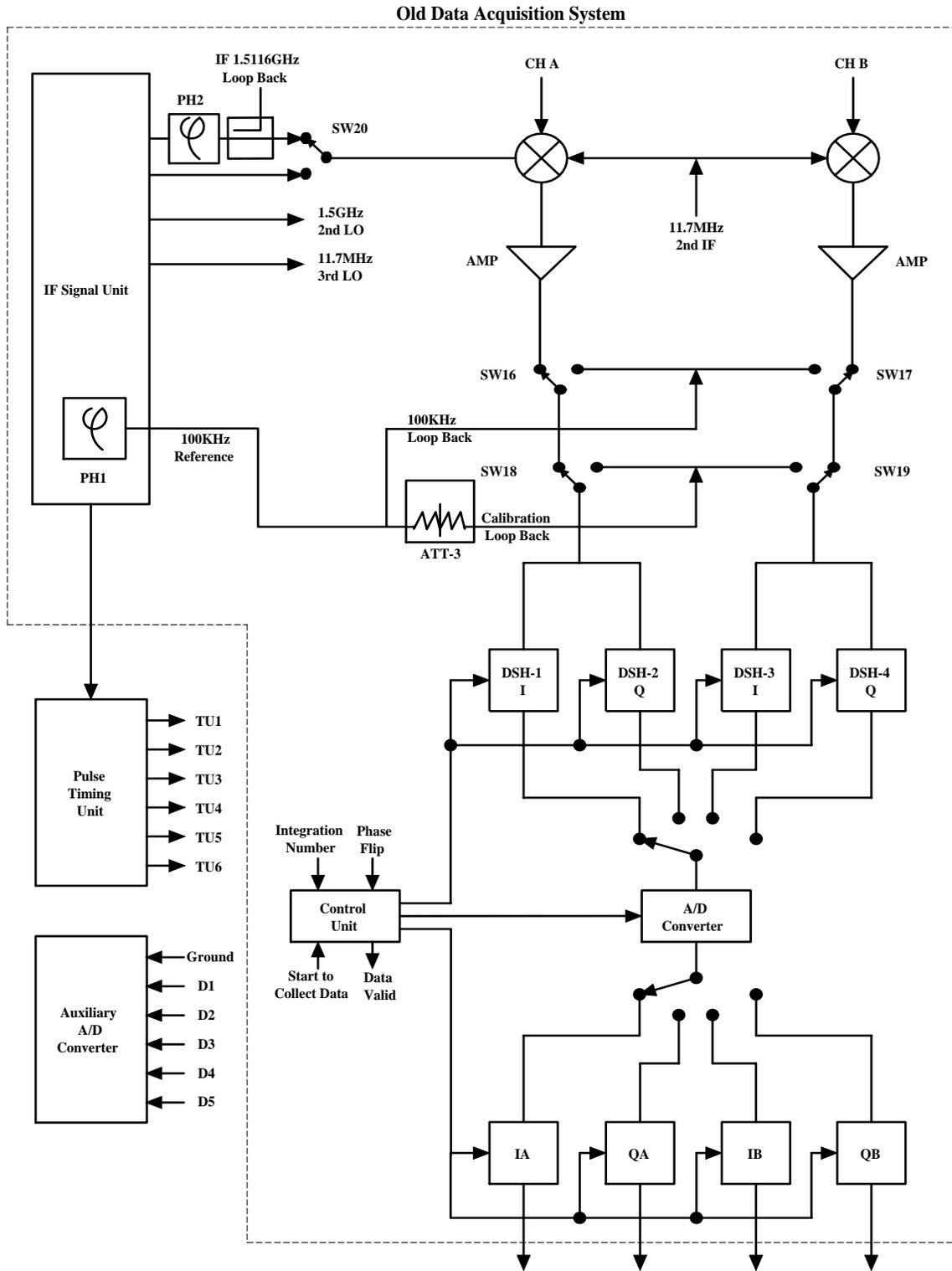
Figure 3.2: The old DAS System Diagram
