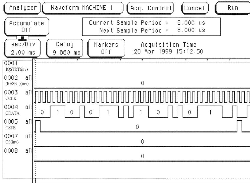
Figure 5.3: Control Words during Transmission
