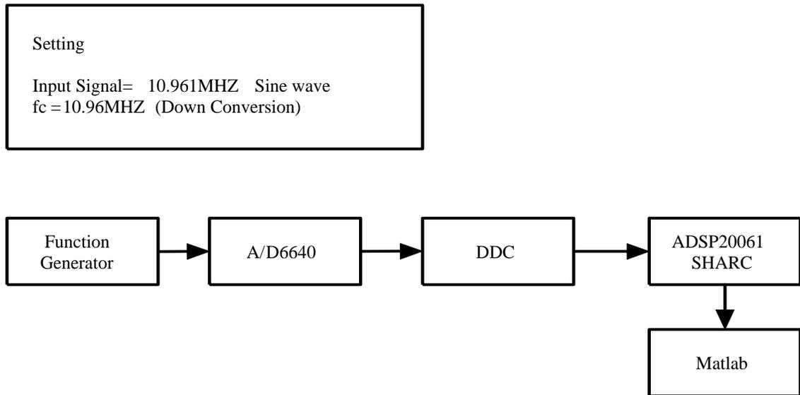
Figure 5.1: The setting of the testing system
