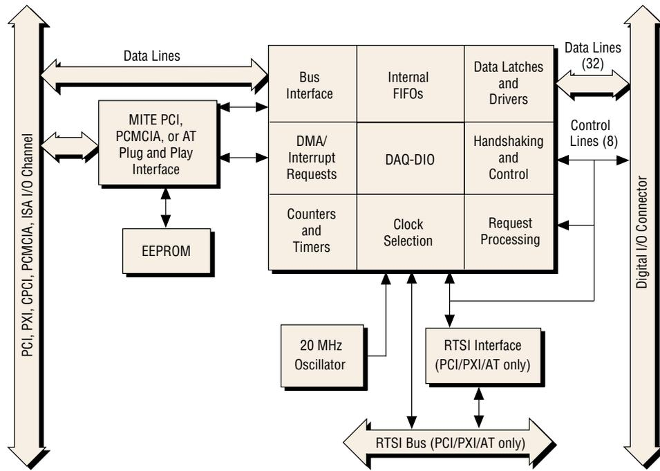
Figure 3.12: PCI-DIO-32HS Block Diagram
