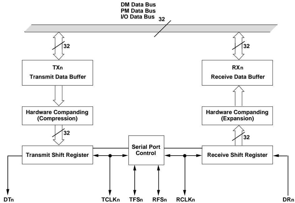
Figure 3.10: Serial Port Block Diagram
