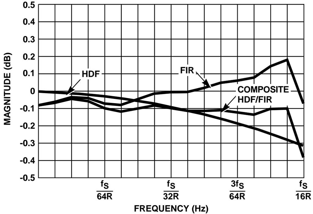
Figure 4.2: Frequency Response of the Composite Filter for R=16
