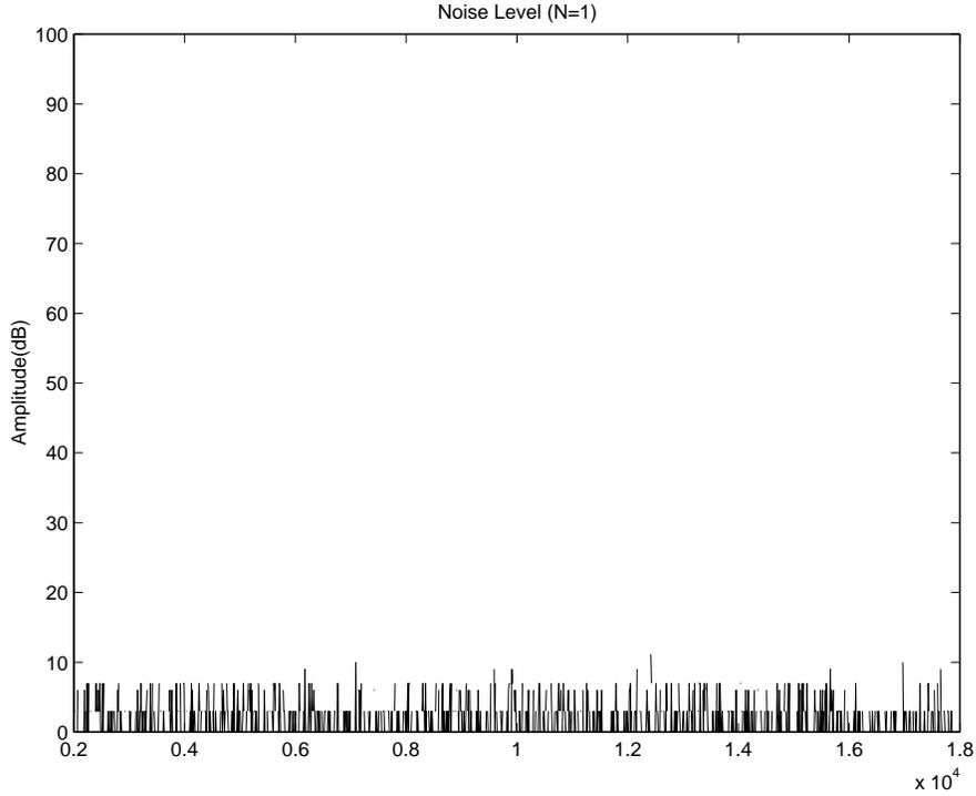
Figure 5.7: Noise Level of the Digital Receiver (N=1)
