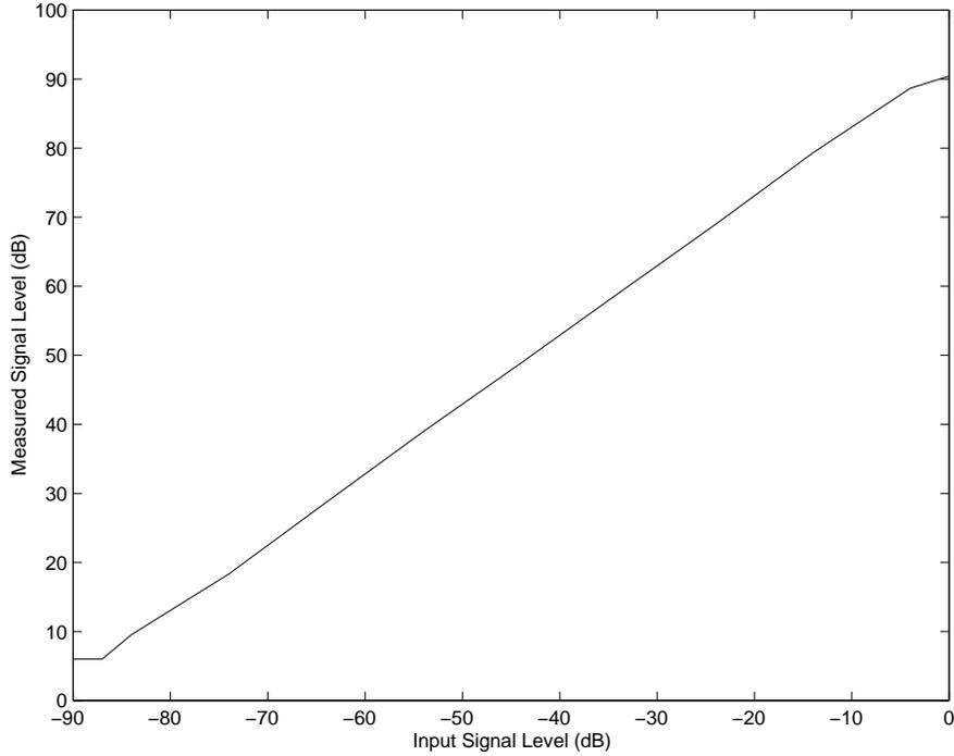
Figure 5.9: Test of the Dynamic Range of the Receiver (N=8)
