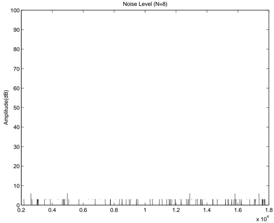
Figure 5.8: Noise Level of the Digital Receiver (N=8)
