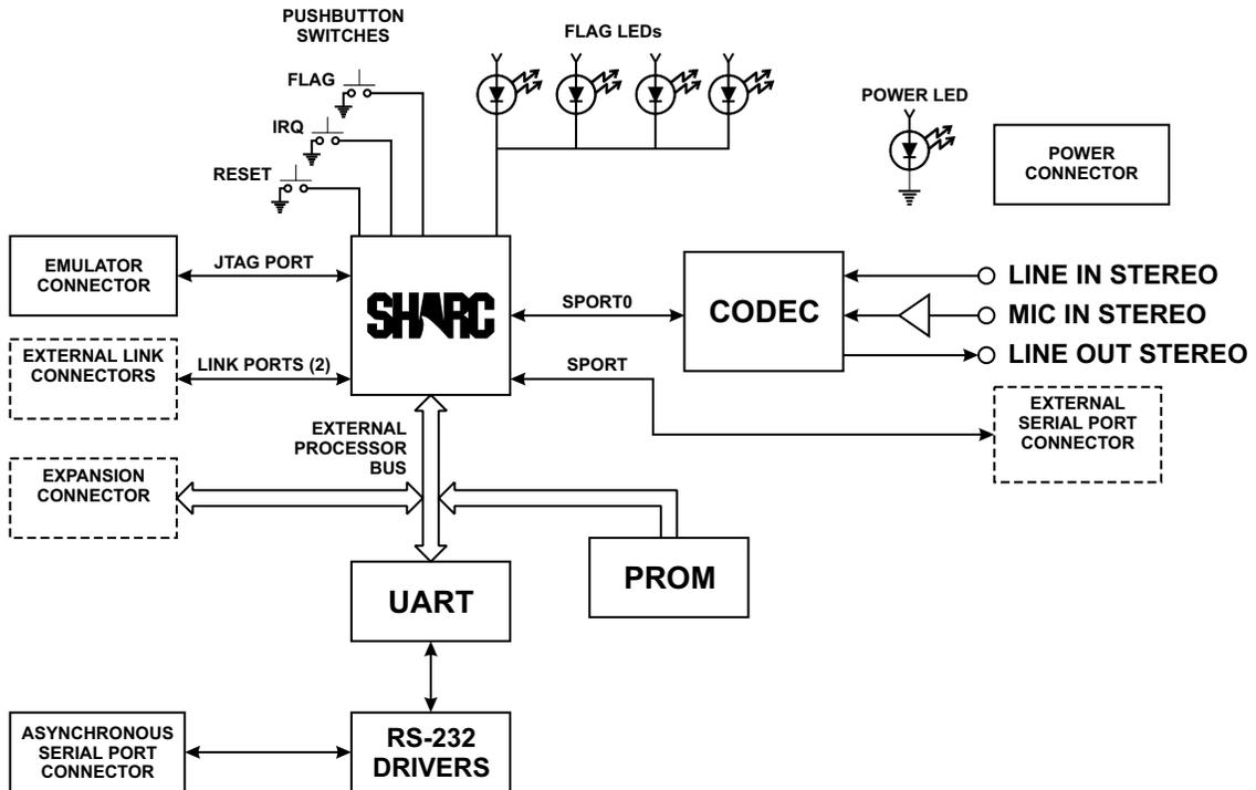
Figure 3.9: SharC Board System Block Diagram
