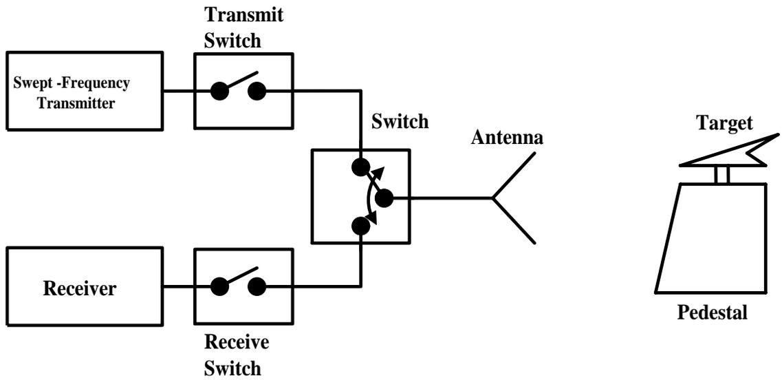
Figure 2.3: A pulsed RCS measurement system
