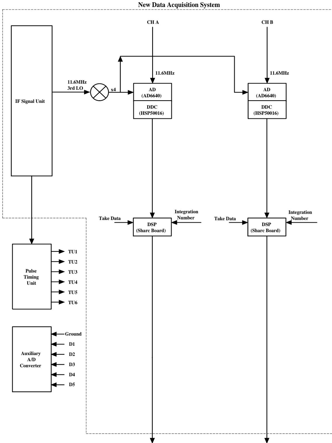
Figure 3.3: The new DAS System Diagram
