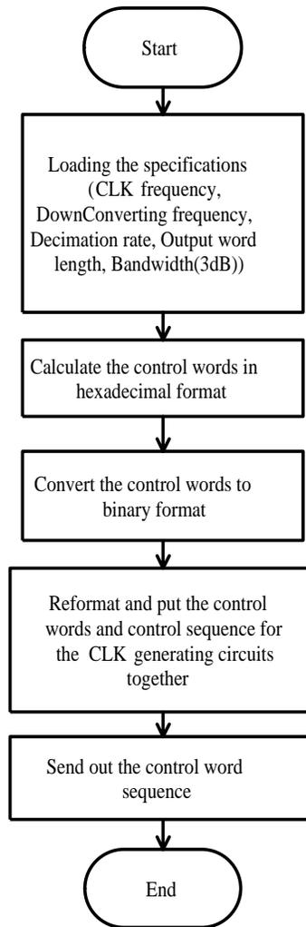
Figure 4.4: Flow Diagram of the Control Word Generator
