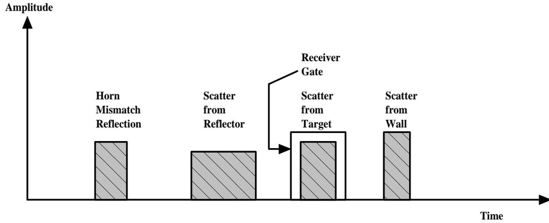
Figure 2.4: Compact range system timing diagram
