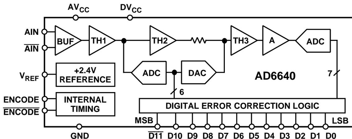
Figure 3.4: The Functional Block Diagram of AD6640
