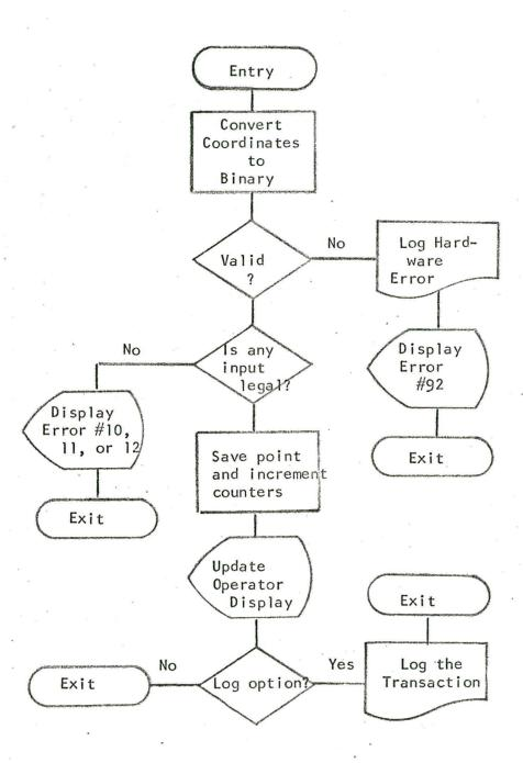
TYPICAL COMMAND PROCESSING -The "ERASE POINT" Service Routines
