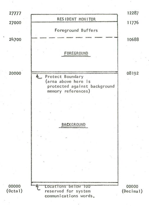
This diagram shows the location of the various components of our system in the memory of the DDP-116 computer.
