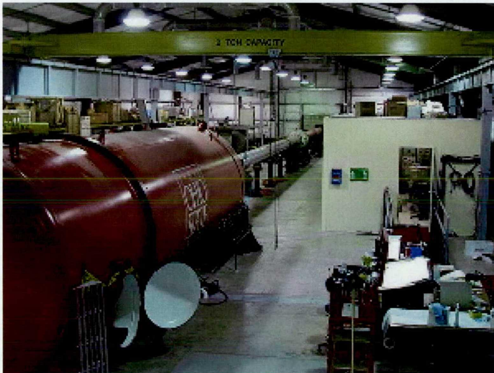
Figure 26. Shock tube facility (TTF) at the OSU GTL
