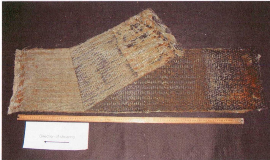
Figure 4.26: Failure surface for a hydrated W/NW NP GCL specimen after cyclic and static shearing.
