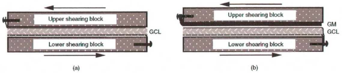
Figure 2.11: Direct shear configurations illustrating end-clamping for (a) GCL internal and (b) GM/GCL interface shear tests (Fox and Stark 2004).
