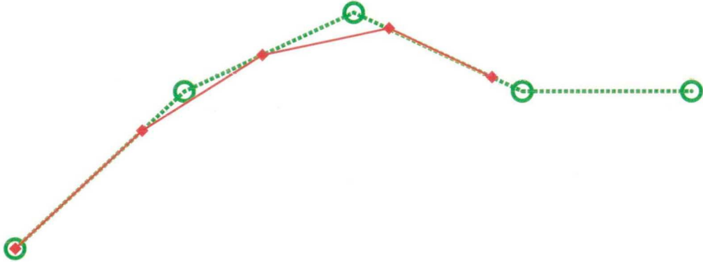
Figure 3.8: While undergoing contraction, the basis grid points do not penetrate any deeper than the line segments joining their initial positions. In this example, the open points represent the initial positions and the filled points represented the contracted positions. The points have been contracted by 25%.
