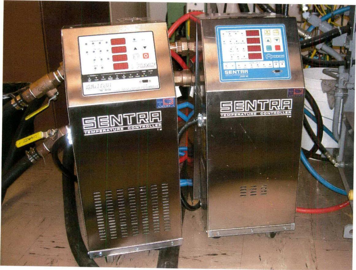
Figure 3.7: Temperature controllers used to control the mold temperature.
