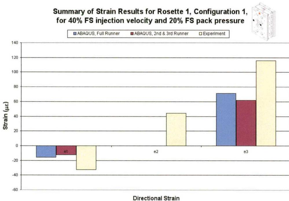
Figure 5.9: Strain gage rosette one results comparison for configuration one (µε) for 40% FS injection velocity and 20% FS pack pressure.
