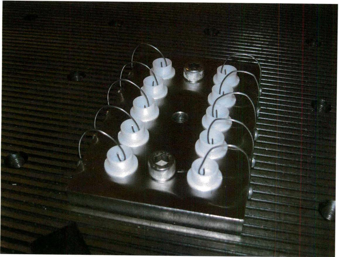
Figure 5.22: CMM jig used to fixture parts during measurement.
