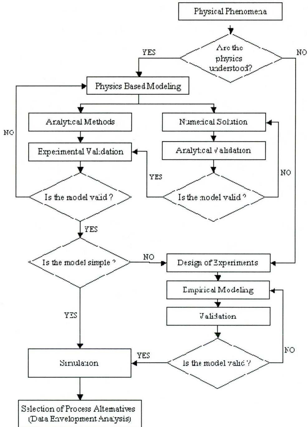
**Figure 2.1:** Process Modeling Scheme [6]
