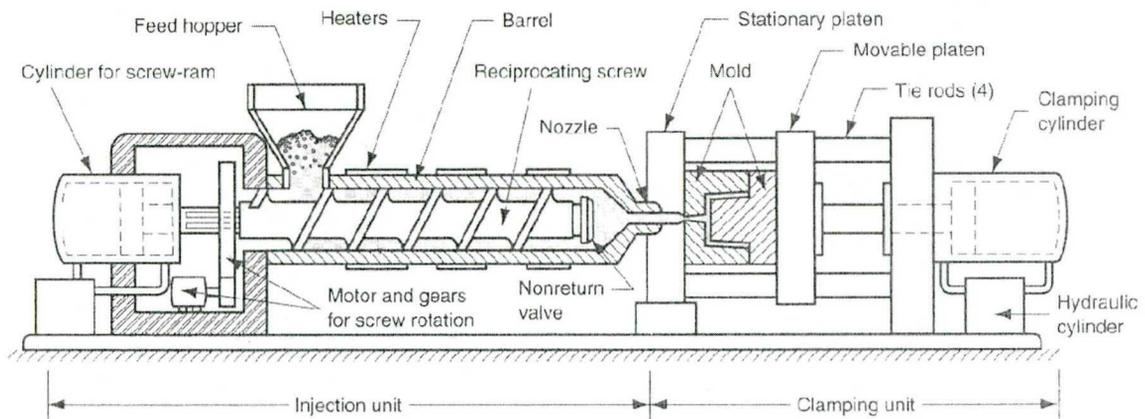
**Figure 1.1:** Typical injection molding machine [3]
