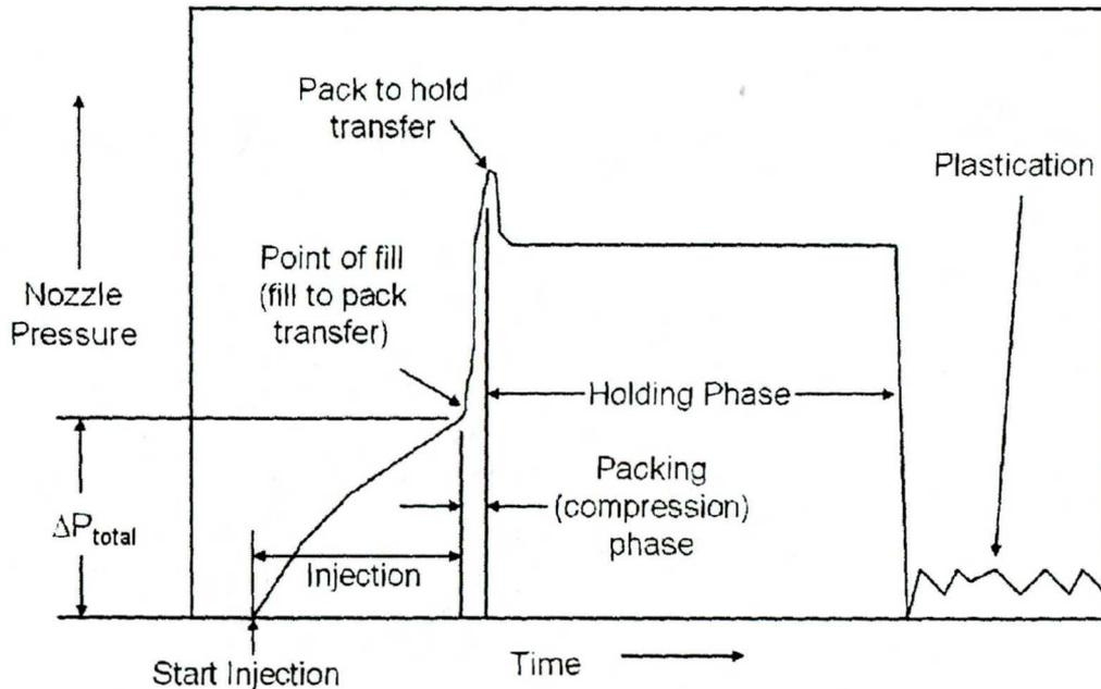
**Figure 1.2:** Pressure at the injection location for one cycle of IM [4]
