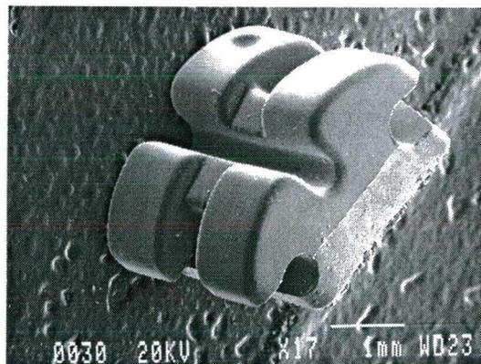
**Figure 26.** SEM photograph of a Contour bracket: Archwire slot edge.
