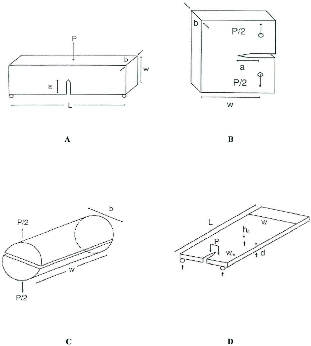
**Figure 2.** Specimen geometries for the determination of fracture toughness: Single-edge notched method (A) (Lloyd and Adamson, 1987); compact tension method (B) (Kovarik *et al.*, 1991); short rod with chevron notch method (C) (Pilliar *et al.*, 1986); double torsion method (D) (Goldman 1985).
