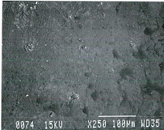
**Figure 12.** SEM photograph of the surface of a Contour bracket (*as received*).
