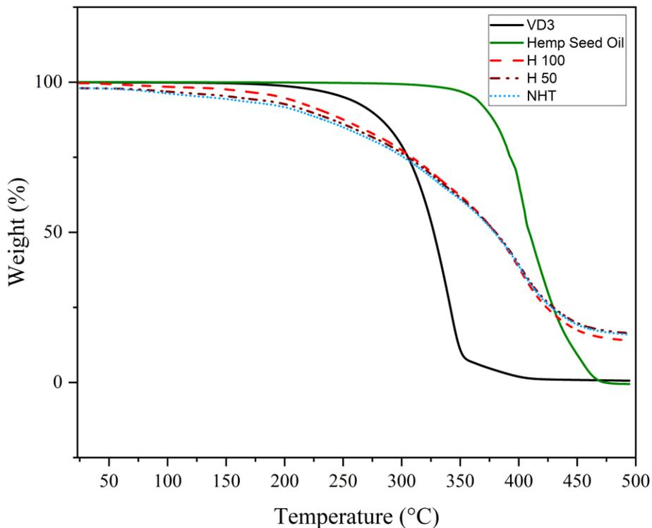
Figure 4.5: Thermogravimetric curve for Vitamin D3, Hemp seed oil and encapsulated vitamin D3 samples
