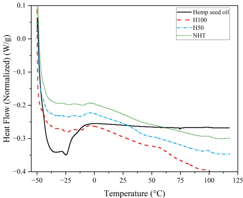
Figure 4.7:DSC thermograms for hemp seed oil and encapsulated VD3 samples
