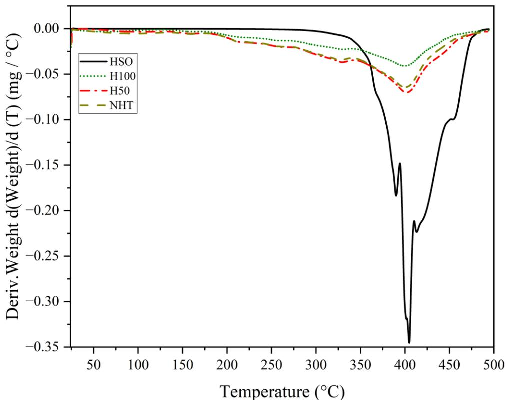
Figure 4.6: Derivative thermogravimetric (DTG) curve for Hemp seed oil and encapsulated vitamin D3 powders
