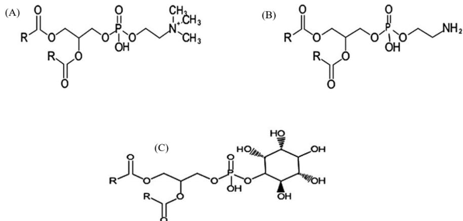
Figure 2.2: Structure of commonly observed Phospholipids in soybean lecithin. (A) Phosphatidylcholine, (B) Phosphatidylethanolamine, (C) Phosphatidylineositol
