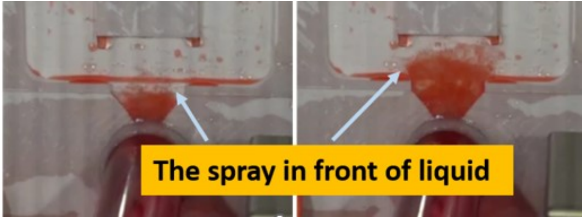
Figure 1.2: The spray effect observed in water analog experiments.
