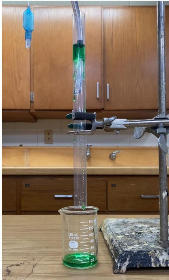
Figure 8.2. Benchtop setup of the apparatus during a PVC cuff leak test.
