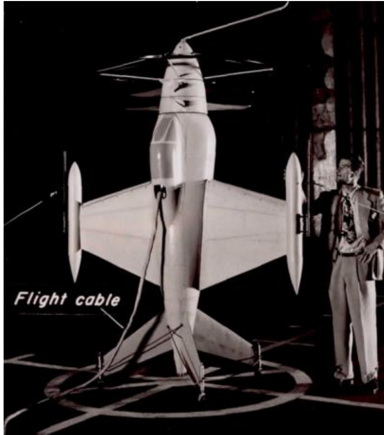
Figure 4: Photograph of a 25% scale model of the XFV-1 aircraft [20].
