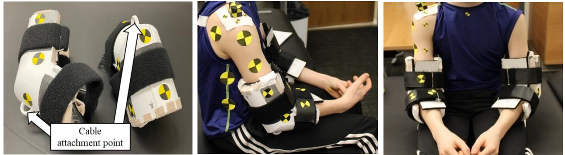
Figure 3: Elbow braces with cable attachment point
