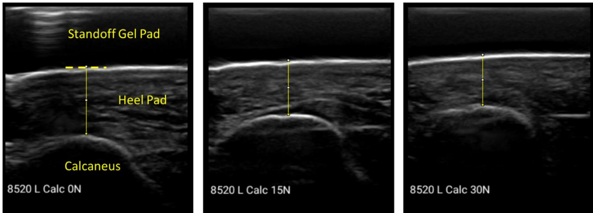
Figure 17: Example Ultrasound Measurements of Left Calcaneus: 0 N (left), 15 N (middle), and 30 N (right). The dotted line shows the outermost layer of the skin.
