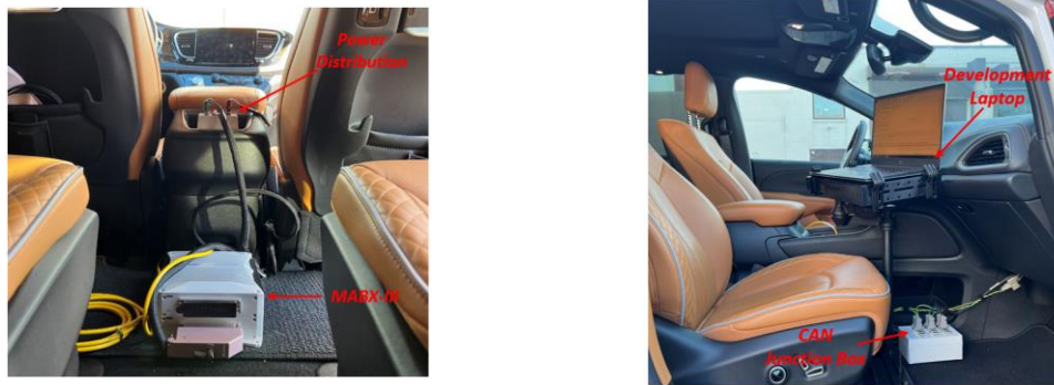
Figure 2.10: Installation of the MABX-III connection to CAN
