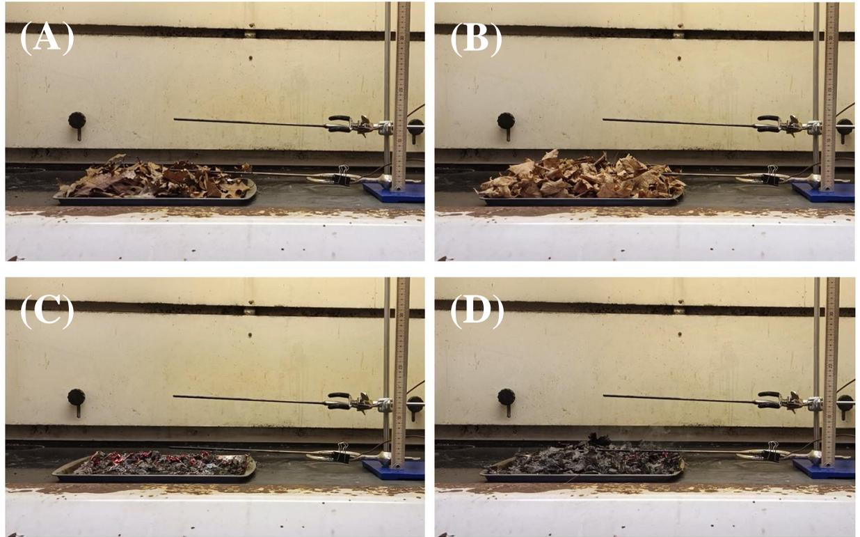
Figure 3.2 Fuel sample ignition experiment. (A) prior to burning with oak sample, (B) prior to burning with maple sample, (C) post-burn with oak sample, (D) post-burn with maple sample.
