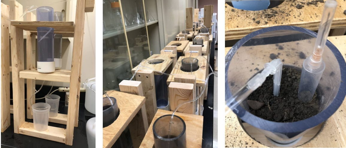
Figure 3 Laboratory setup showing the soil column (left), irrigation system (center), and syringe used for air testing (right)
