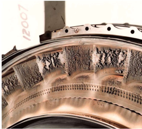
Figure 2: Volcanic ash deposits on turbine NGVs from British Airways Flight 9 [4]
