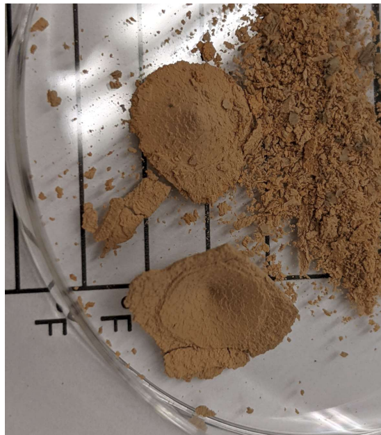
Figure 32: An ARD central deposit split in two, parallel to cone surface, revealing layered structure of cone
