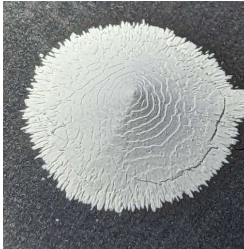
Figure 30: Close up of an albite deposit at 1033K plate surface temperature showing the wavefronts of layer formation
