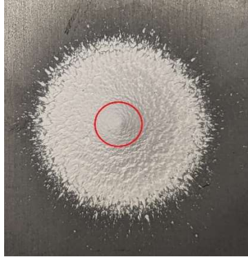
Figure 24: Representative alumina deposit at 1144K plate surface temperature
