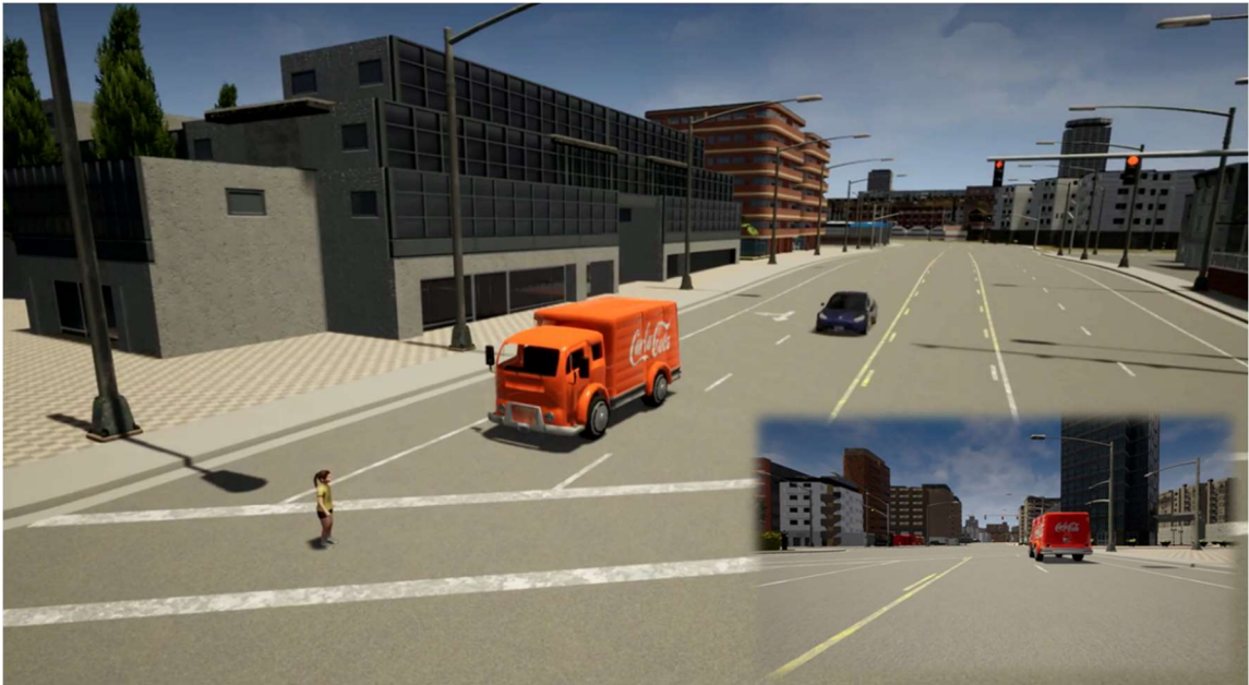
Figure 13 Right bottom foreground: Host vehicle camera image, Background: scenario image from an external camera showing view that is obstructed by truck [3].
