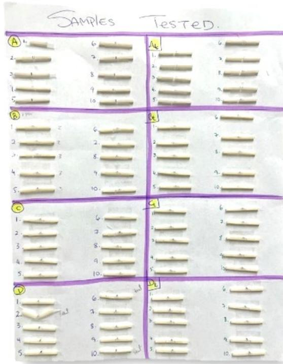
Figure 9. Fractured samples preserved for fracture location analysis under x3.5 magnification.
