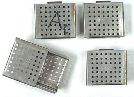
Figure 5. Four metal boxes for thermocycling. Box At had the m-PMMA samples.
