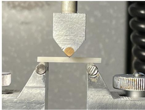
Figure 7. 3-Point-Bending test for FS.
