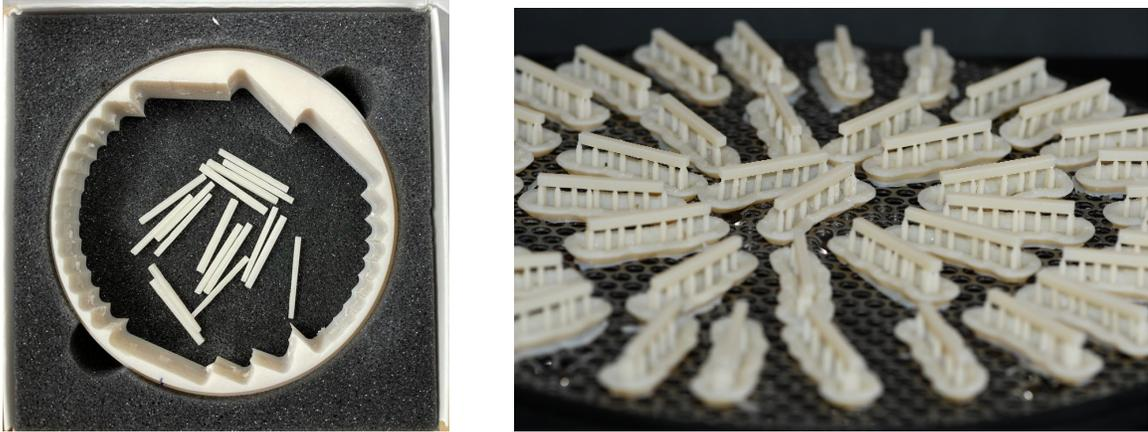
Figure 3. Milled PMMA and 3D-printed UDMA samples.
