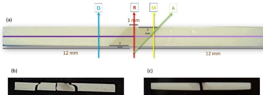
Figure 10. (a) Mode of failure diagram. O: cohesive failure within de original material, R: cohesive failure within de repair material, M: mixed failure, A: adhesive failure. (b) Example of O mode of failure. (c) Example of R mode of failure.
