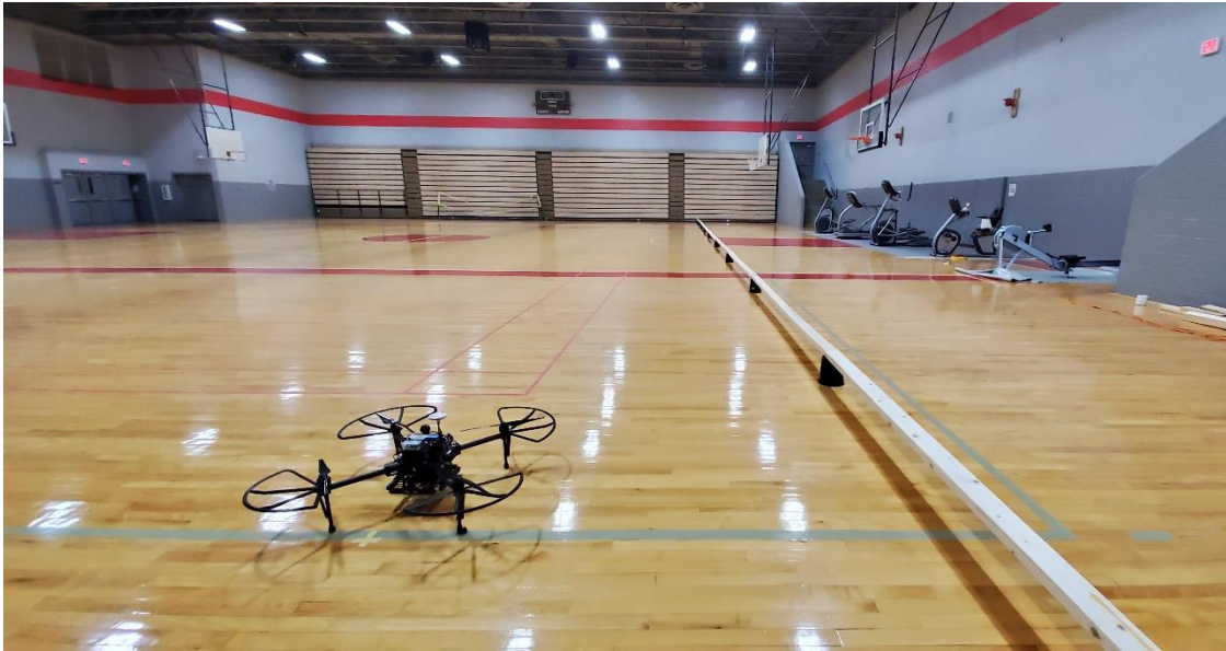
Figure 11. Experimental set for evaluating the accuracy of autonomous flights. The wooden logs were placed along a straight line and elevated from the ground by a set of inverted pots. The UAV was placed adjacent to the logs and flown autonomously, and its relative position from logs was evaluated to calculate the drift under varying speeds. Logs were placed along (a) the width and (b) the length of the test area.
