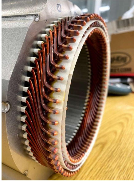
Figure 3. Stator as viewed from the weld side
