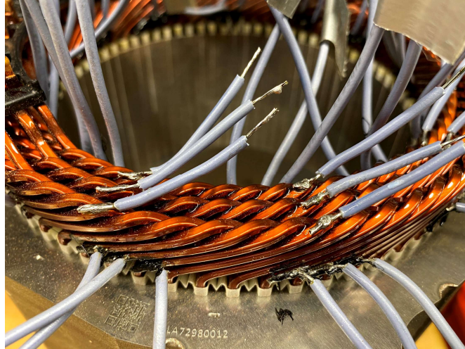
Figure 30. Parallel winding path test connections located on the bend in the coil near the middle of the image compared to the voltage stress testing points located near the bottom of the image closest to the stator core
