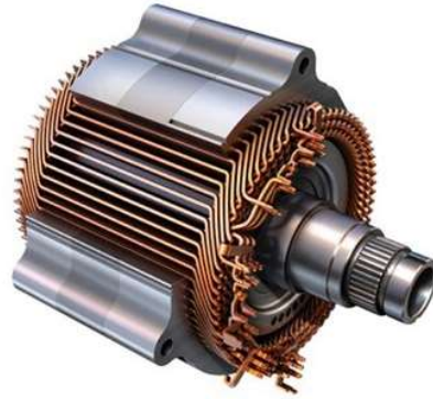
Figure 1. Chevy Bolt traction motor assembly with section view of hairpin windings [15]
