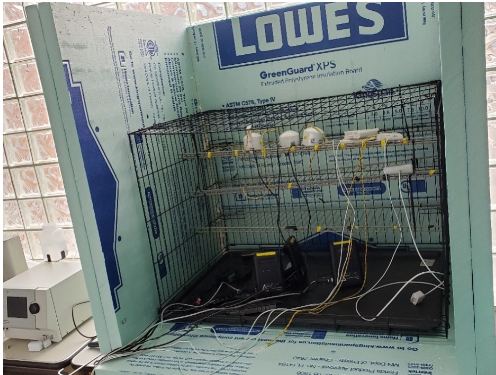
Figure 6.2: Photograph of interior of insulation testing chamber with sensors on racks.
