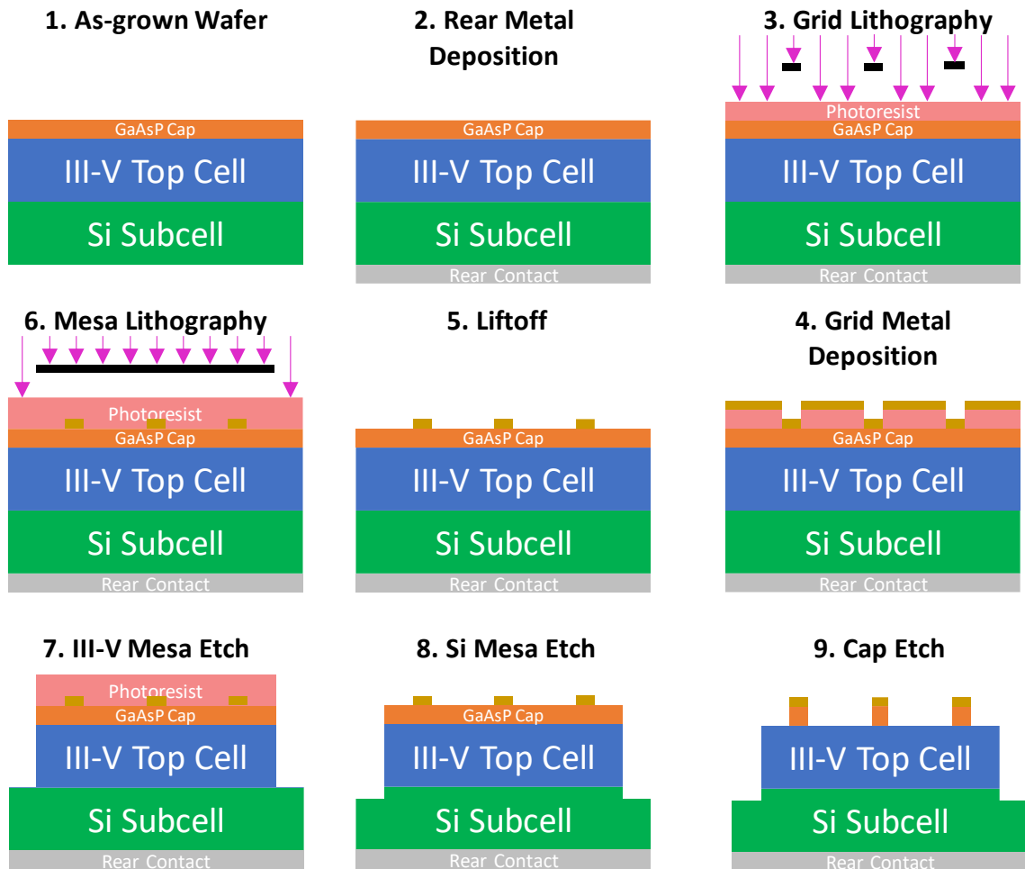
Figure 3.10 Simplified fabrication process flow for a GaAs 0.75 P 0.25 /Si tandem solar cell without and ARC.
