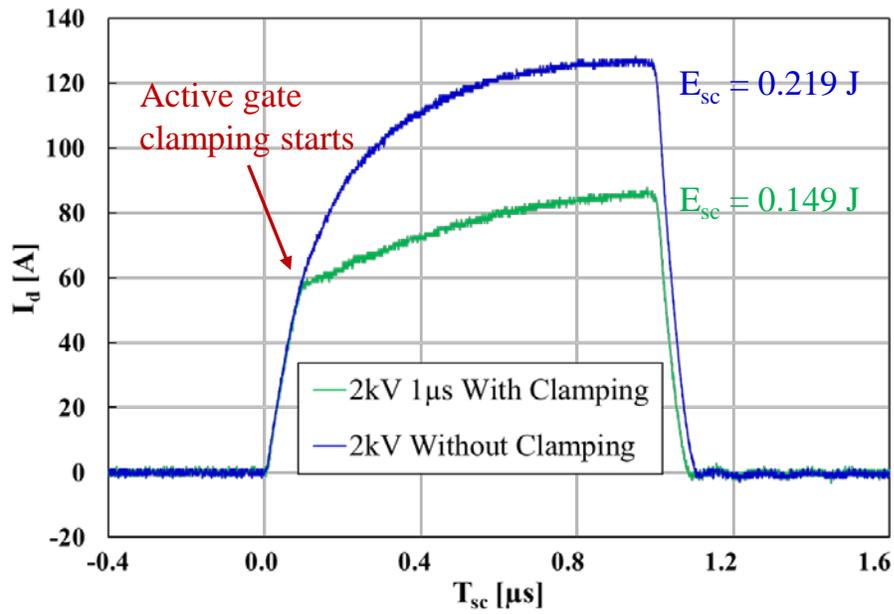
Figure 2.13 Short circuit current comparison with and without gate clamping
