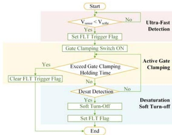
Figure 2.3 Flow chart of the proposed three-step short circuit protection method.
