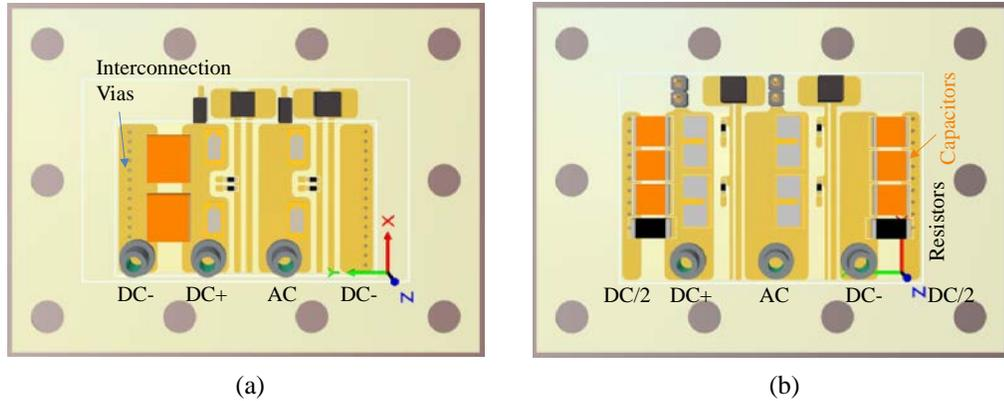
Figure 3.3 DBC vertical power loop layout (a) 1200 V SiC MOSFET (b) 3300 V SiC MOSFET.
