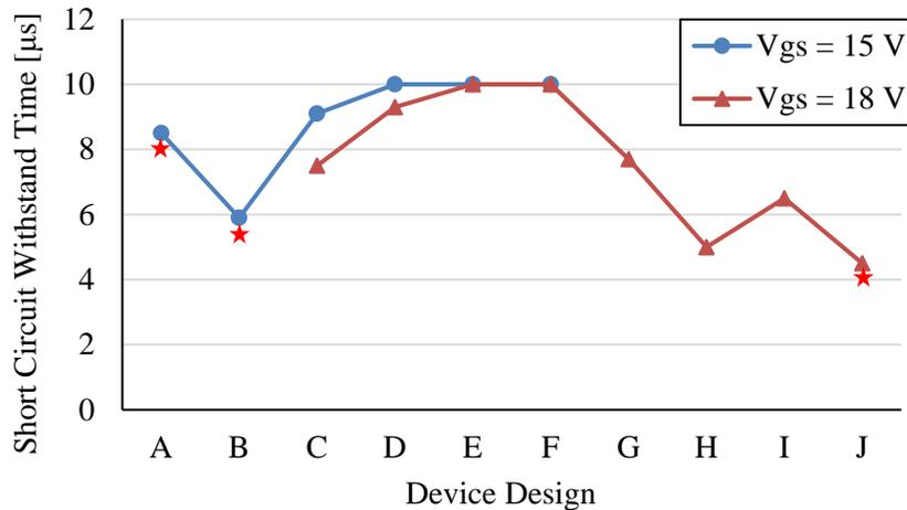
Figure 2.1 3300 V SiC MOSFET short circuit withstand time.
