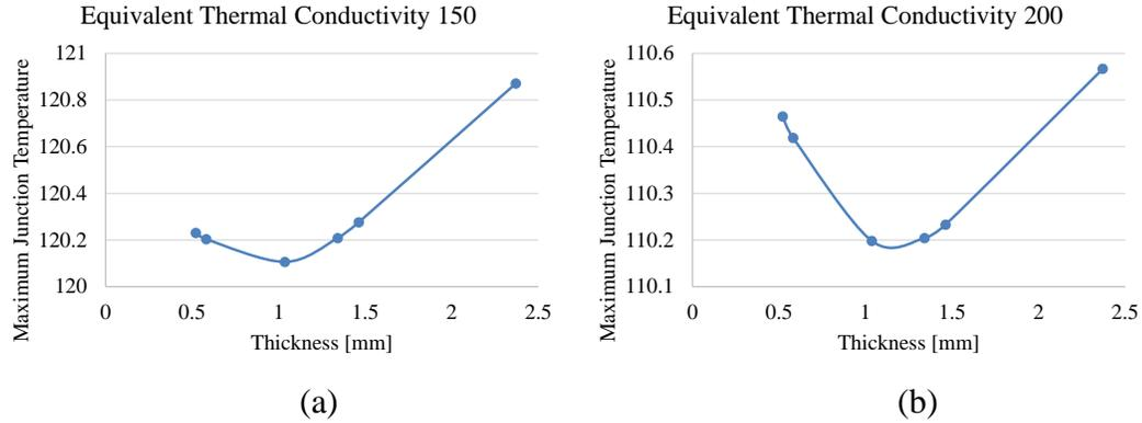
Figure 4.5 Relationship Between Maximum Junction Temperature and DBC thickness
