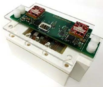
Figure 3.12 Proposed vertical loop based power module assembly with ceramic baseplate and liquid cool housing.
