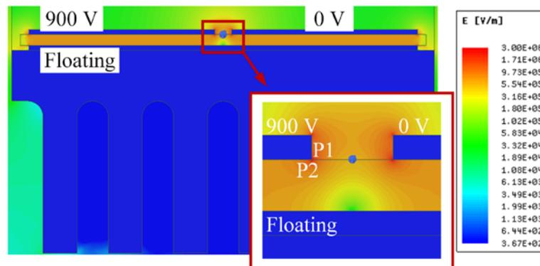
Figure 4.7 Conventional power module structure DM electric field distribution under 900 V.
