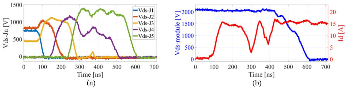
Figure 5.11 Experiment turn-on waveforms of the prototype without voltage balancing capacitors at 2,100 V dc voltage and 15 A load. (a) SCPS drain to source voltage and drain current. (b) drain to source voltage of inner JFETs.
