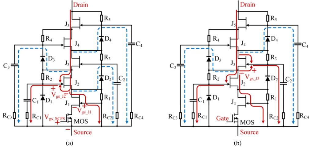
Figure 5.2 The voltage balancing capacitor charging path (a) Stage I, MOSFET and J1 turns off (b) Stage II, J2 to J5 turns off.
