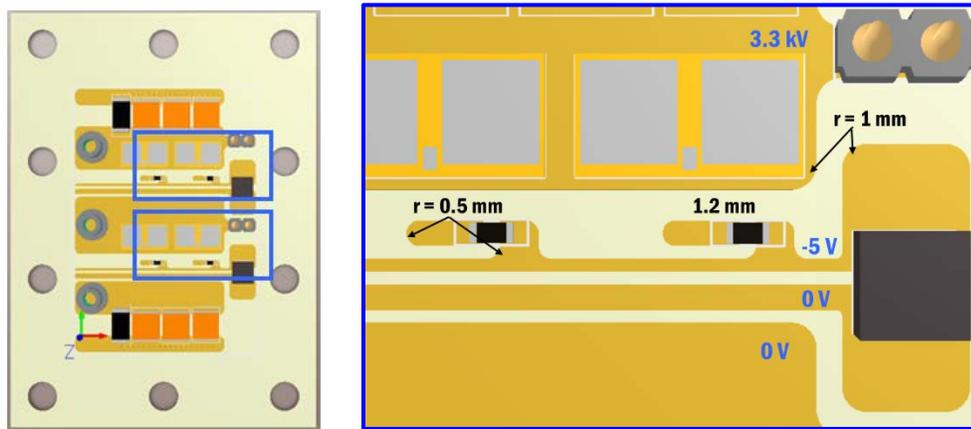
Figure 3.7 3,300 V power module DBC clearance design
