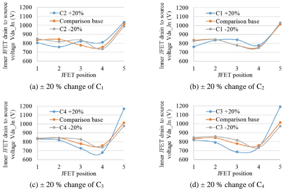
Figure 5.6 Voltage distribution change due to 20 % capacitance change of the voltage balancing capacitors during off state.
