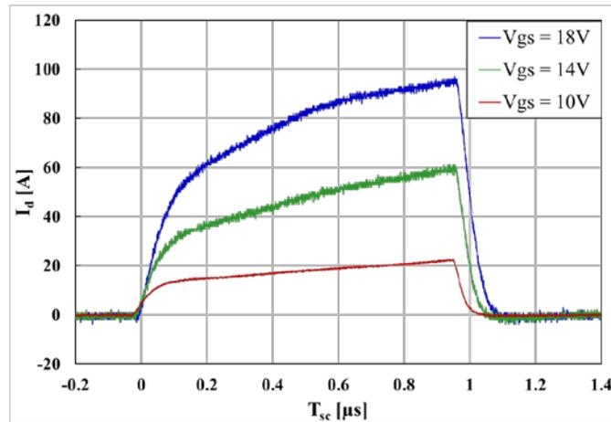
Figure 2.10 Short circuit current under different gate voltages.
