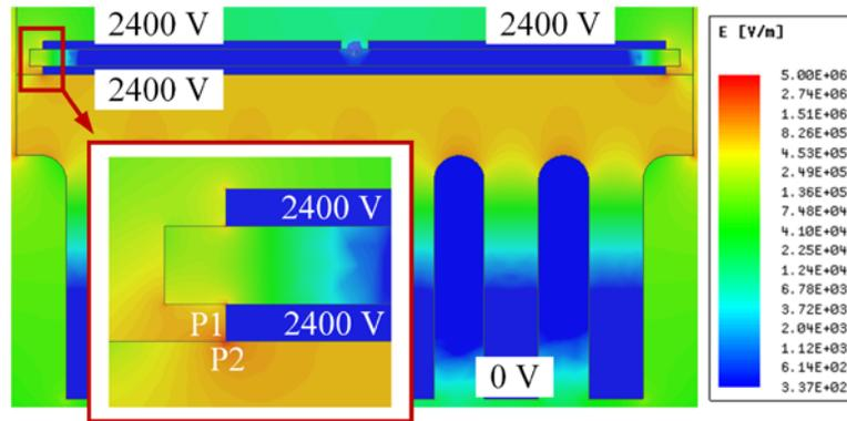
Figure 4.10 Vertical loop power module structure with the ceramic baseplate CM electric field distribution under 2,400 V.
