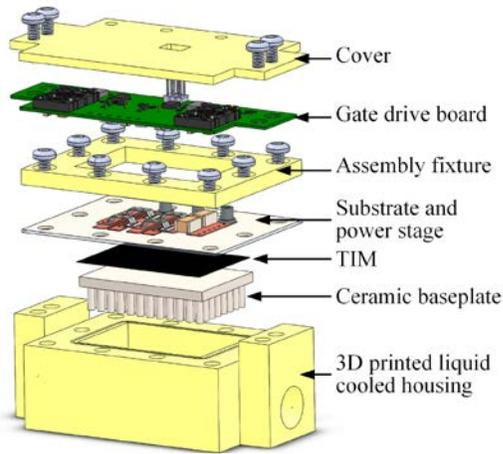
Figure 4.19 Liquid cooled power module assembly design.
