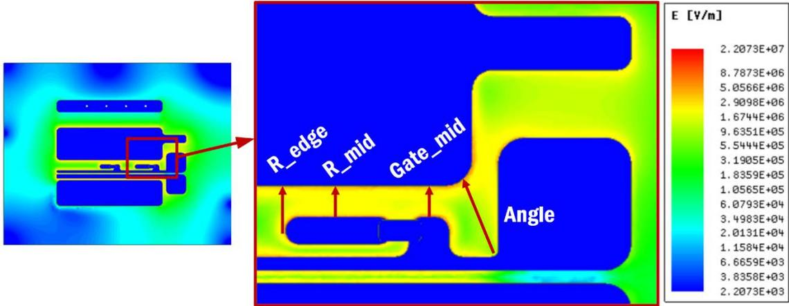
Figure 3.8 3,300 V power module DBC electric field stress distribution
