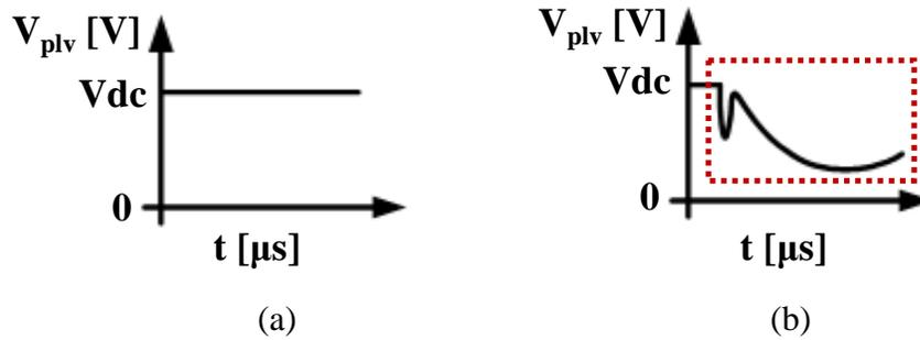
Figure 2.5 Three-step short circuit protection detection signal (a) under normal operation (b) under short circuit condition.
