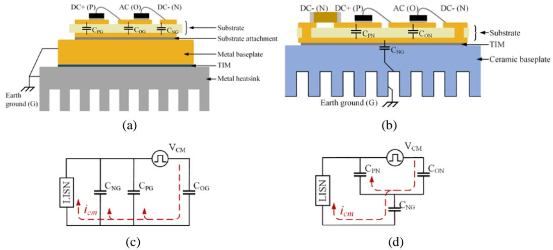
Figure 4.15 Package parasitic capacitance distribution and CM equivalent circuits (a) the parasitic capacitance in the conventional structure (b) the parasitic capacitance in the proposed structure (c) the CM equivalent circuit of the conventional structure (d) the CM equivalent circuit of the proposed structure
