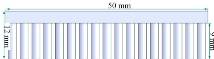
Figure 4.2 Dimensions of the pin fin baseplate
