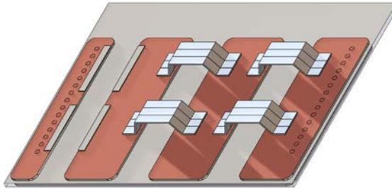
Figure 3.10 Power Loop Parasitic Inductance Extraction Model
