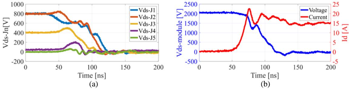
Figure 5.12 Experiment turn-on waveforms of the prototype with optimized voltage balancing capacitors at 2,100 V dc voltage and 15 A load. (a) SCPS drain to source voltage and drain current. (b) drain to source voltage of inner JFETs.
