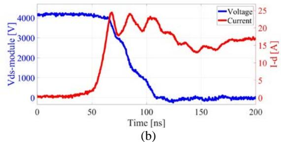
Figure 5.13 Experiment turn-on waveforms of the prototype with optimized voltage balancing capacitors at 4,200 V dc voltage and 15 A load. (a) super-cascode power switch drain to source voltage and current. (b) drain to source voltage of inner JFETs.
