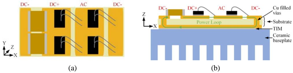
Figure 3.1 Half-bridge power module design with the vertical power loop layout (a) the top view of DBC layout (b) the side view of the power module structure.
