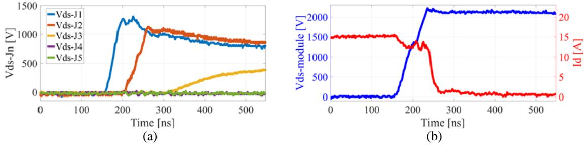
Figure 5.9 Experiment turn-off waveforms of the prototype without voltage balancing capacitors at 2,100 V dc voltage and 15 A load. (a) SCPS drain to source voltage and drain current. (b) drain to source voltage of inner JFETs.
