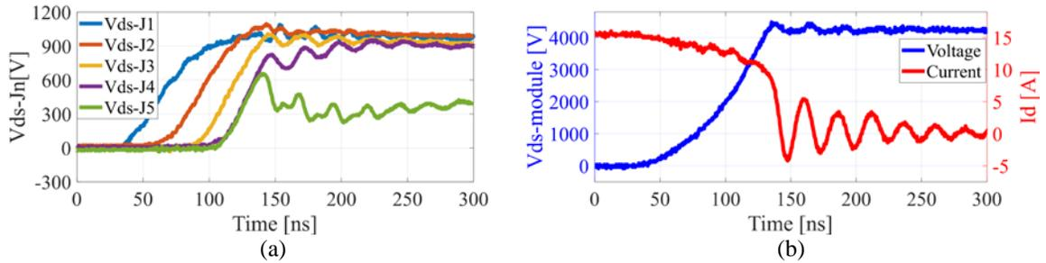
Figure 5.14 Experiment turn-off waveforms of the prototype with optimized voltage balancing capacitors at 4,200 V dc voltage and 15 A load. (a) super-cascode power switch drain to source voltage and current. (b) drain to source voltage of inner JFETs.
