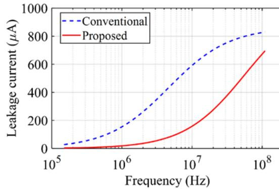
Figure 4.18 Comparison of the CM leakage current under varying frequency.
