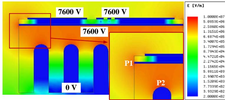
Figure 4.14 Vertical loop power module structure with AlN baseplate CM electric field distribution under 7,600 V.
