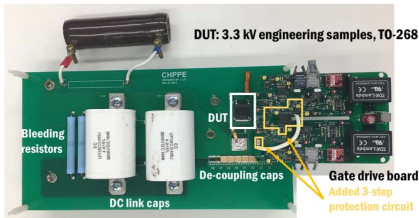
Figure 2.8 3300 V SiC MOSFET short circuit protection evaluation board
