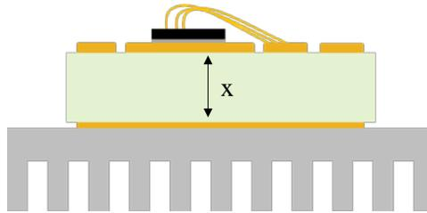
Figure 4.4 Thermal Simulation Model for DBC Thickness Impact
