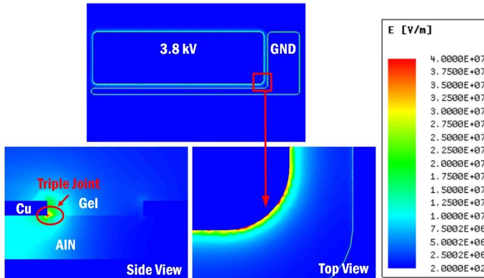
Figure 3.6 Electric field distribution of the DBC sample with 3.8 kV voltage excitation
