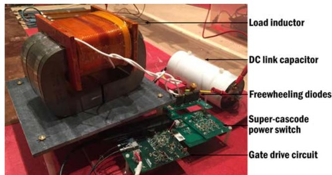
Figure 5.8 The 4,500 V super-cascode power switch double pulse test setup.
