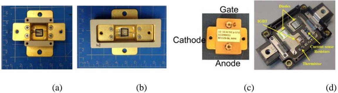
Figure 1.5 Package for quick prototype package for medium voltage SiC power devices
