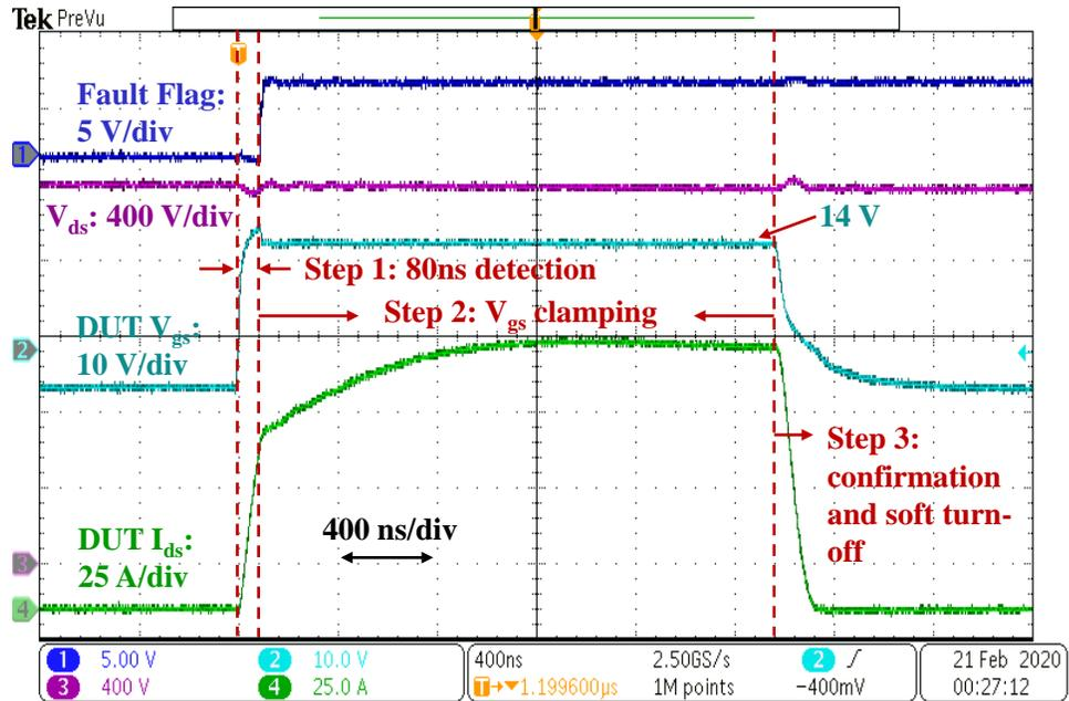
Figure 2.12 3300 V SiC MOSFET three-step protection waveform
