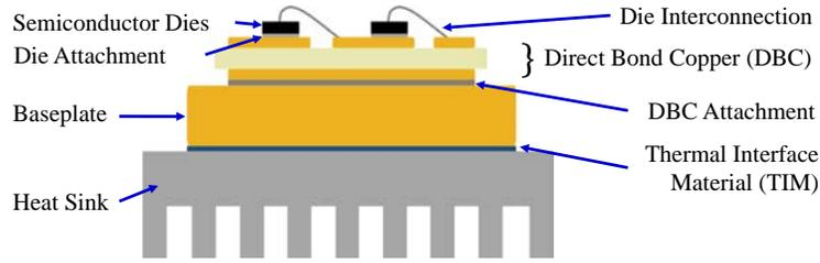
Figure 4.1 The Conventional Power Module Structure
