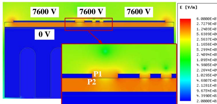
Figure 4.12 Conventional power module structure CM electric field distribution under 7,600 V.
