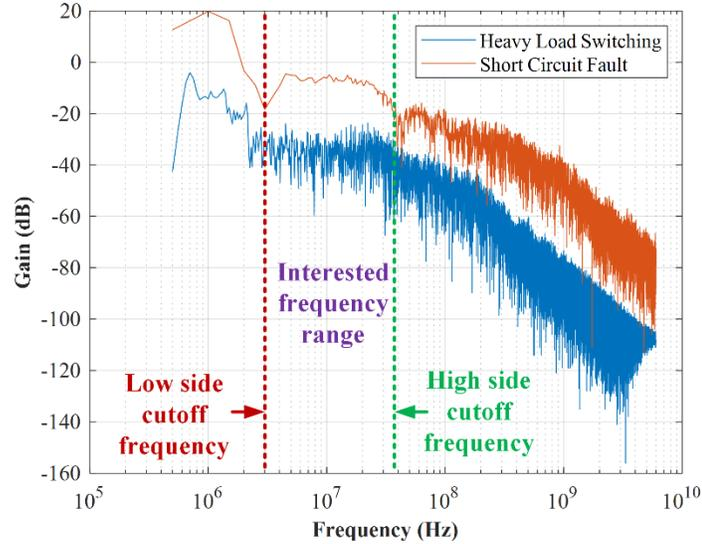
Figure 2.7 Detection circuit design: FFT analysis of  $V_{plv}$  for detection circuit filter design.
