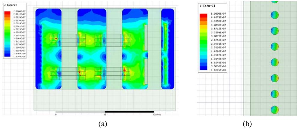
Figure 3.11 Current Distribution (a) across the Cu Trace (b) through Interconnection Vias
