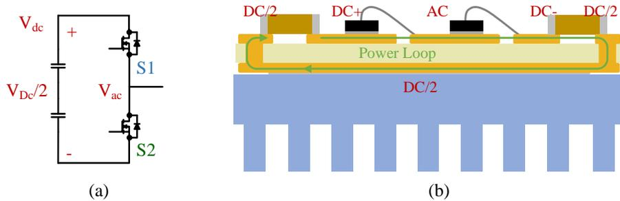
Figure 3.2 Half-bridge power module design with the vertical power loop layout (a) equivalent circuit (b) the side view of the power module structure.
