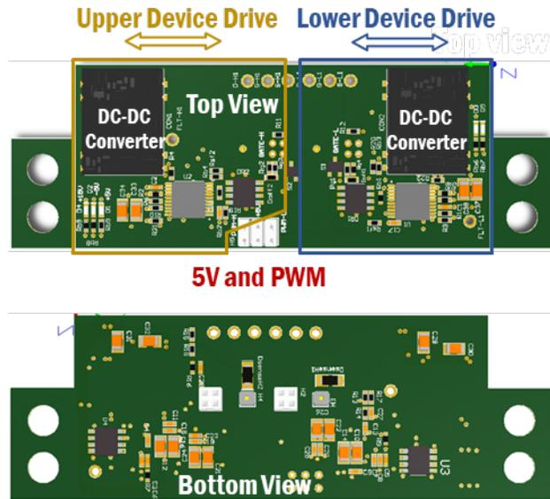
Figure 4.20 Integrated gate drive board design.
