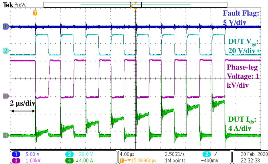
Figure 2.14 Noise immunity test under different load current.
