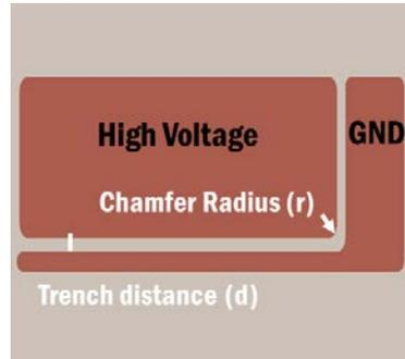
Figure 3.4 DBC sample design illustration
