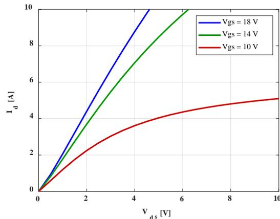
Figure 2.11 3300 V SiC MOSFET I-V curve
