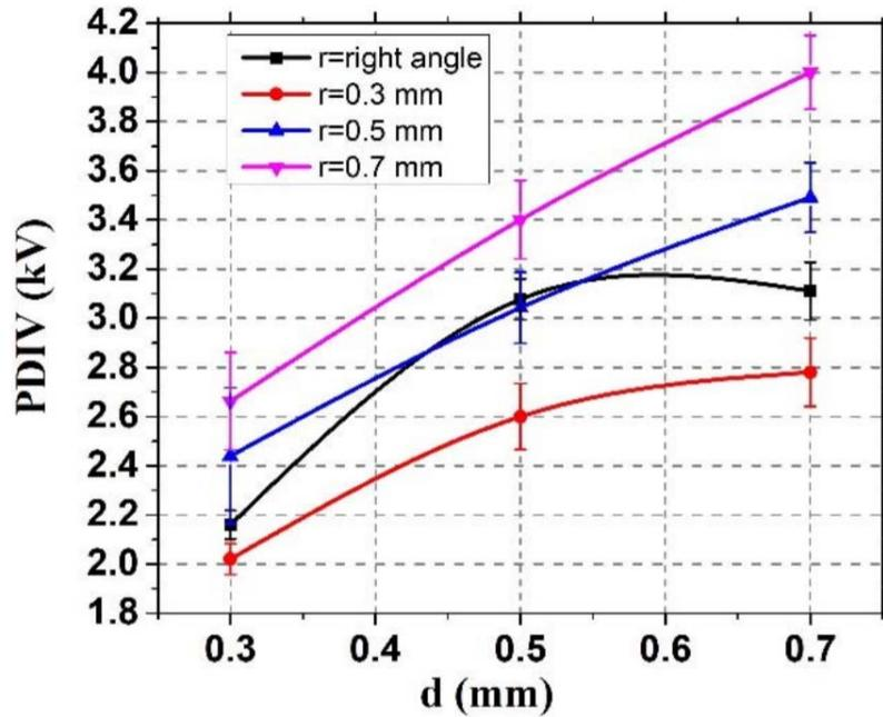
Figure 3.5 The relationship between PDIV, trench distance  $d$  and chamfer radius  $r$
