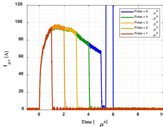
Figure 2.9 3300 V SiC MOSFET short circuit withstand time
