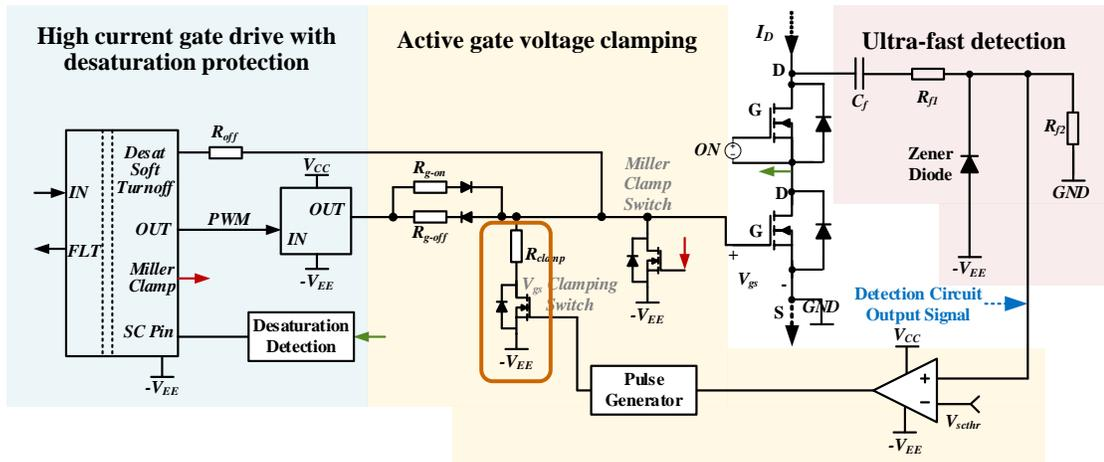
Figure 2.2 Diagram of the proposed three-step short circuit protection circuit.
