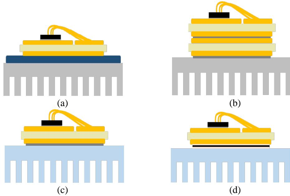
Figure 4.3 Four Power Module Structures with Al and AlN pin fin baseplates
