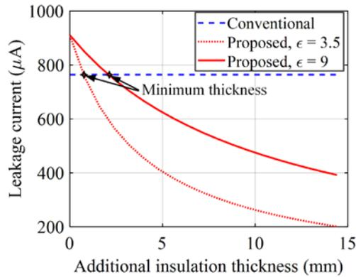
Figure 4.17 Comparison of the CM leakage current with different insulation materials under varying insulation layer thicknesses.
