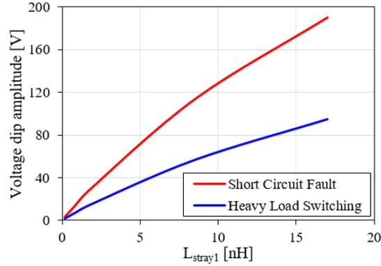
Figure 2.6 Relationship between  $L_{stray1}$  and the target voltage dip amplitude.
