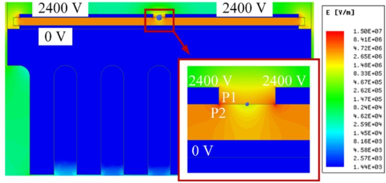
Figure 4.8 Conventional power module structure CM electric field distribution under 2,400 V.
