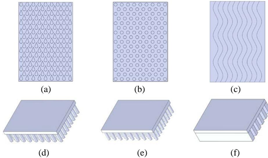
Figure 4.6 Ceramic baseplate designs for comparison
