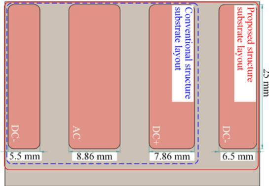
Figure 4.16 Dimensions of the substrate layout
