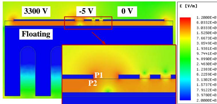
Figure 4.11 Conventional power module structure DM electric field distribution under 3,300 V.
