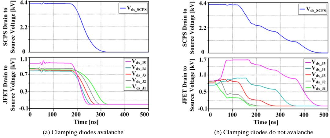
Figure 5.4 Simulated SCPS and JFET drain to source voltage during the turn-on transient
