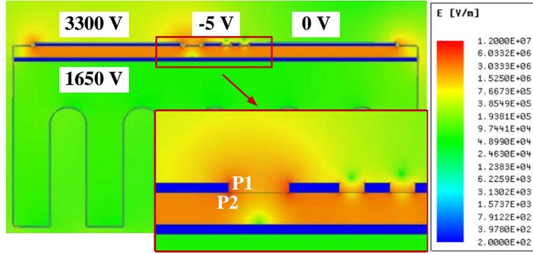
Figure 4.13 Vertical loop power module structure with AlN baseplate DM electric field distribution under 3,300 V.
