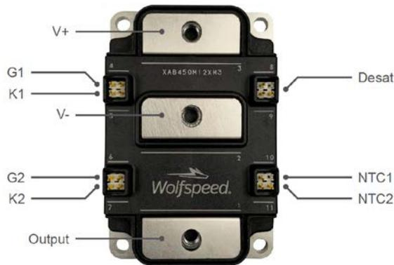
(a) External package and pinout
