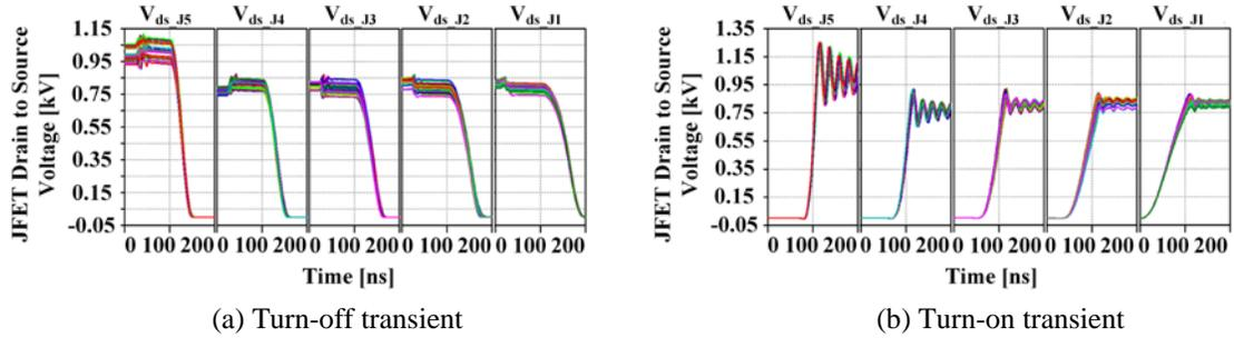
Figure 5.7 Switching waveforms under selected voltage balancing capacitor tolerance.
