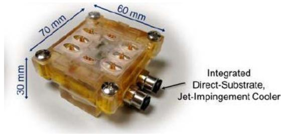
Figure 1.8 Integrated jet-impingement cooling in the SiC device packaging
