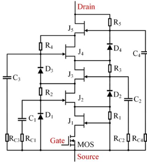
Figure 5.1 The super-cascode structure
