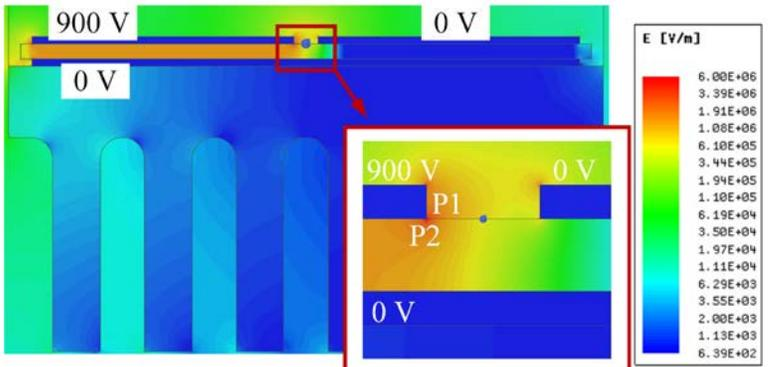
Figure 4.9 Vertical loop power module structure DM electric field distribution under 900 V.
