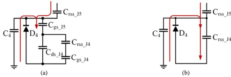
Figure 5.5 Current path during turn-on transient (a) in equivalent circuit (b) in simplified equivalent circuit.
