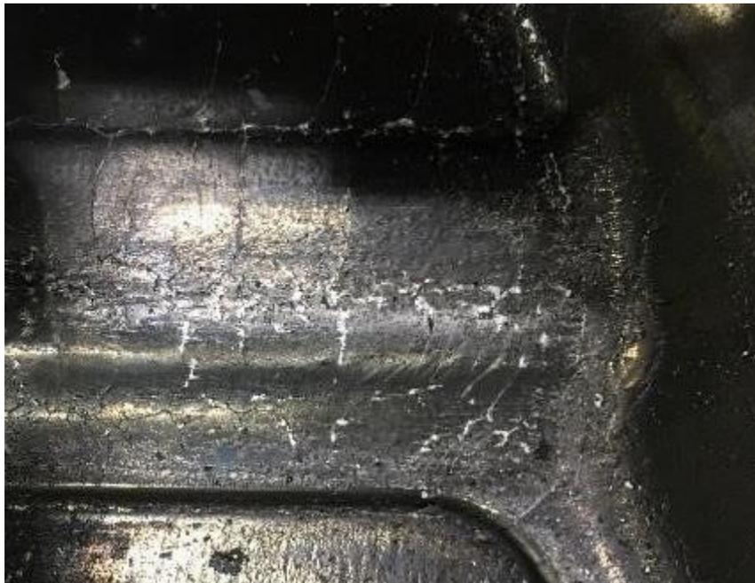
Figure C1: Damage on a HPDC Die Surface
