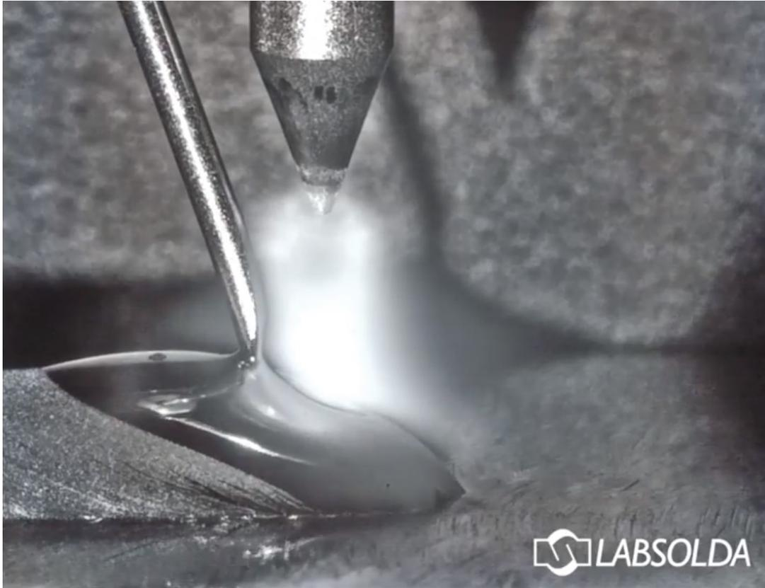
Figure A2 : Uninterrupted Bridging Metal Transfer in Rear Feed Cold Wire GTAW (5)
