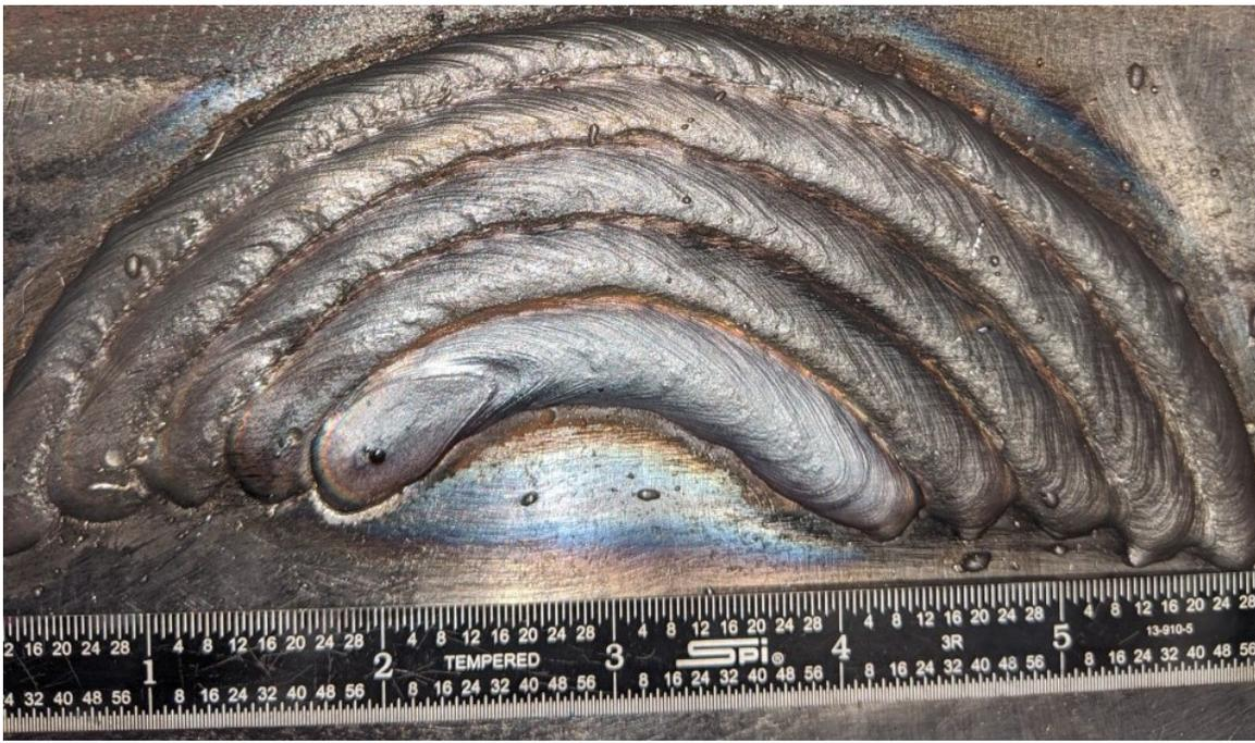
Figure B14 : Multi-Pass Anviloy Wire Clad on H13
