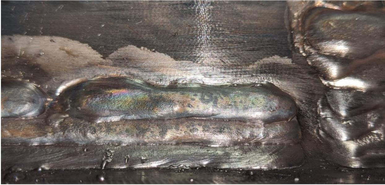
Figure B18 : Horizontal (2G) Welds with Refined Oscillation
