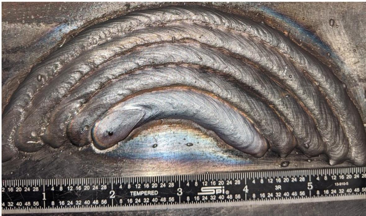
Figure 22 : Multi-pass 1G Robotic GMAW Clad Procedure
