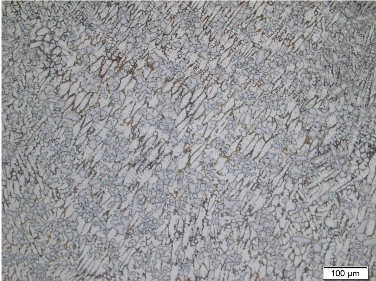
Figure D25 : Normalized & Double Tempered Anviloy Wire – H13 Clad Fusion Zone
