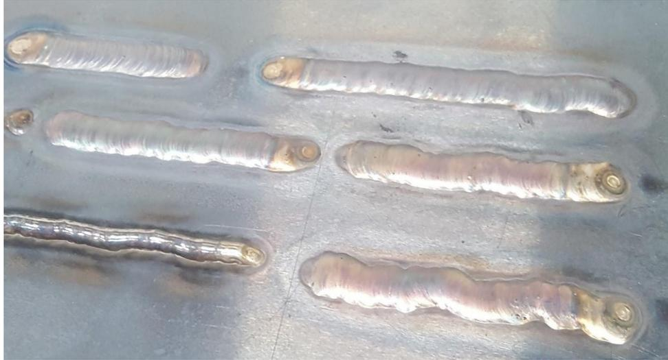
Figure A5 : GTAW Welds From OSU Capstone Group (3)
