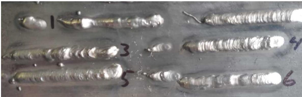
Figure A10 : Welds Made with Two Axis Wire Straightener
