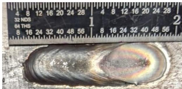
Figure 21 : Weld Using the DC- Wave 1.2mm SuS waveform at 260A Using Oscillation
