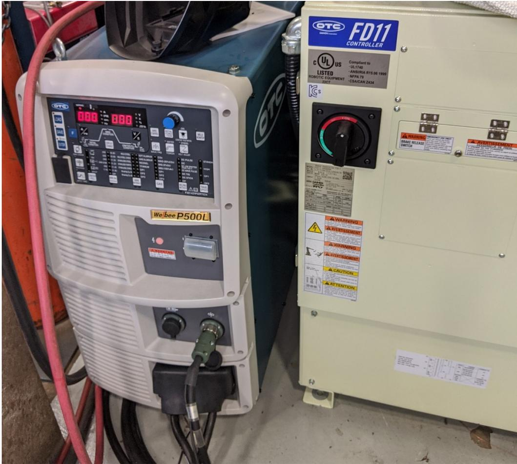
Figure B8 : OTC Robot Controller and OTC Welding Power Supply
