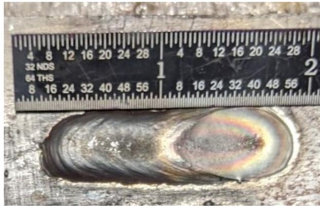
Figure B13 : Oscillation Adjusted Flat (1G) Weld
