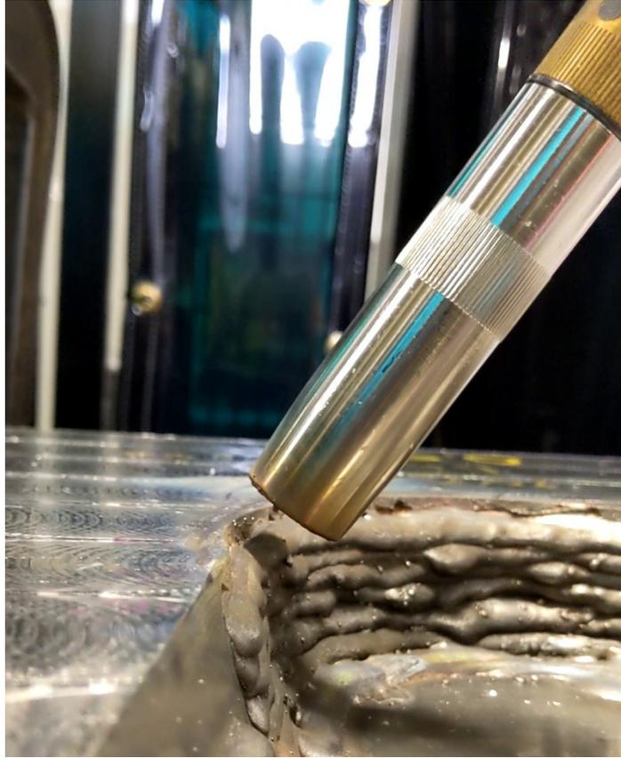
Figure B15 : Torch Angle for Horizontal Welds
