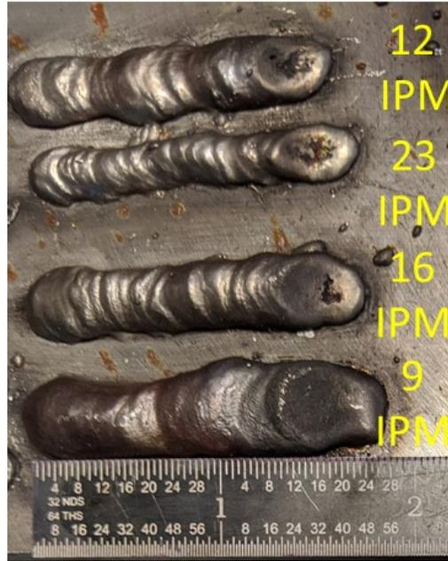
Figure 19 : 1G GMAW Synchrofeed Welds Showing Lack of Fusion
