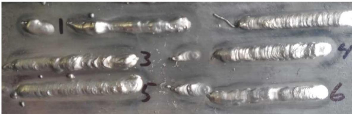
Figure 16: CW-GTAW Welds Made Without Wire Straightener (Top) Vs. Early Development HW-GTAW Welds Made with Wire Straightener (Bottom)
