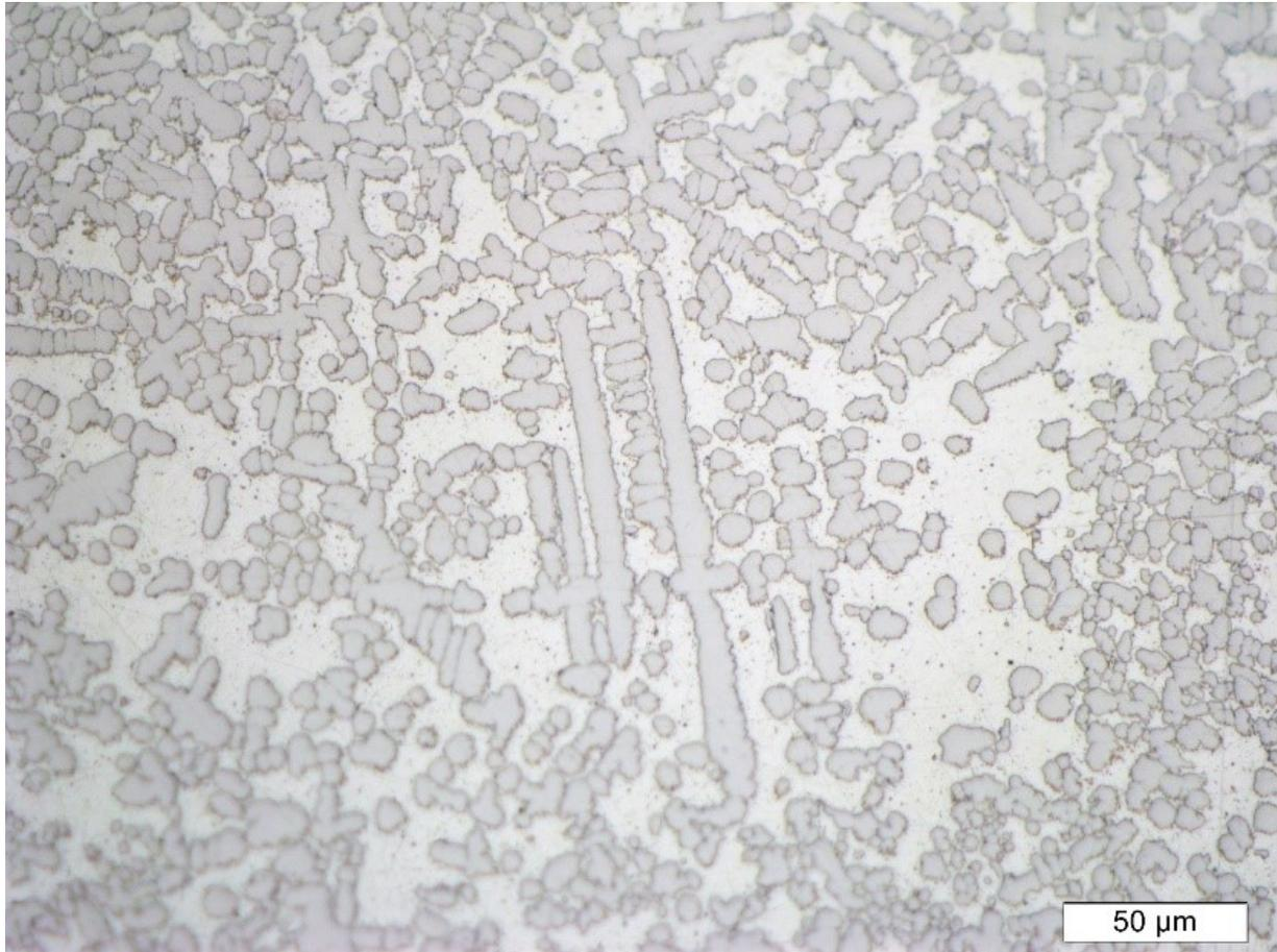
Figure 32 : Metallographic Section of Anviloy Wire Arc Casted Button Showing Undiluted Two Phase Microstructure
