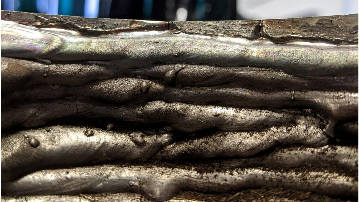
Figure B16 : Initial Horizontal (2G) Welds
