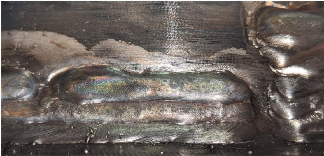
Figure 24 : 2G Position Clads Employing Torch Angle Oscillations
