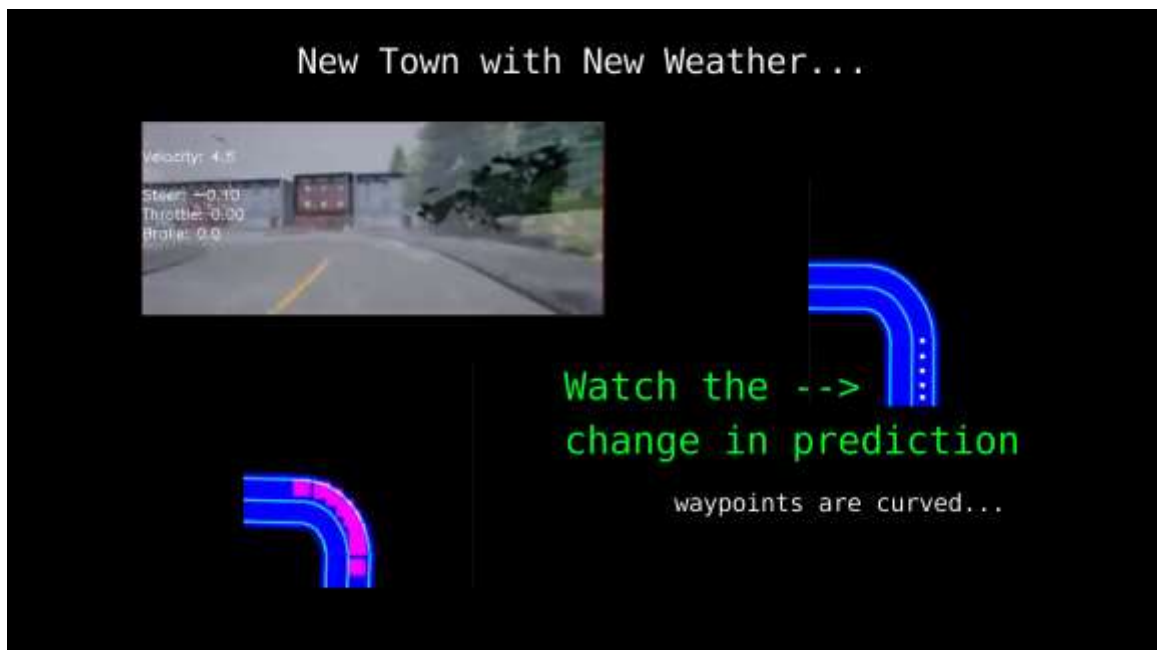
Figure 21: Lane-keeping – cornering (c) – waypoints before turning
