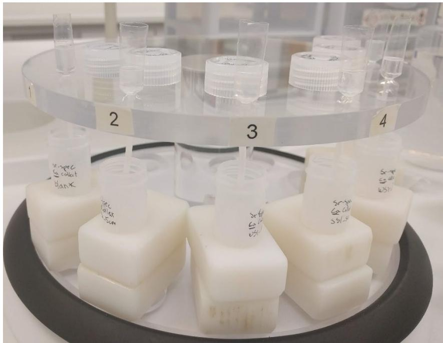
Figure 4-1 Sr-spec columns used for purifying samples.
