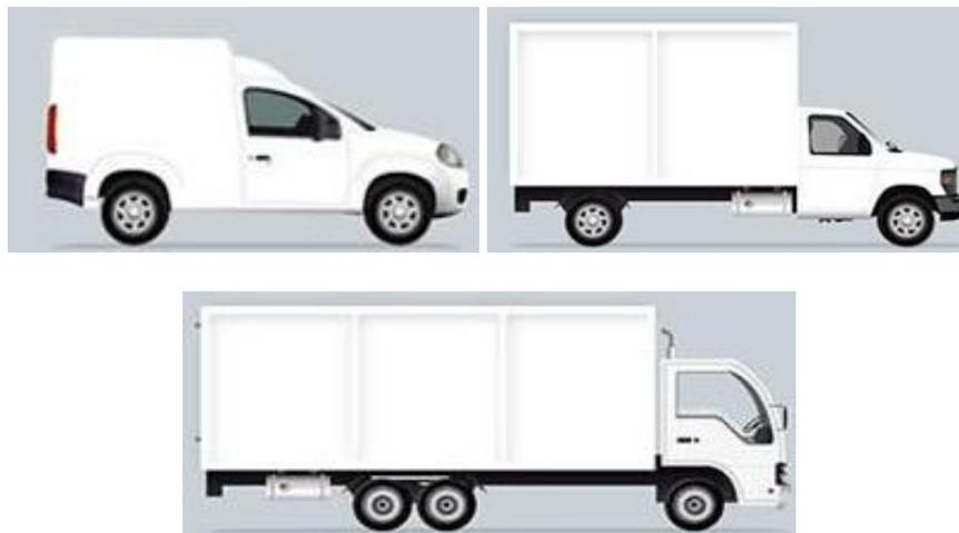
Figure 5: Freight vehicles of category N1, N2 and N3 respectively (data from: Chinese Classification of power-driven vehicles and trailers, GB/T 15089-2001)
