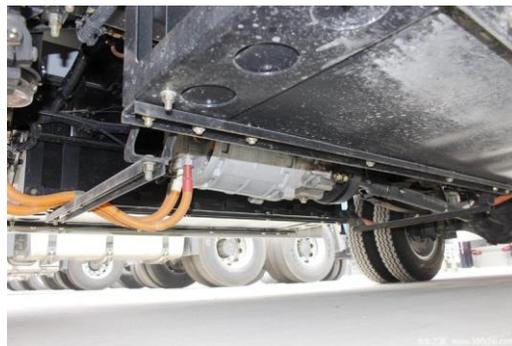
Figure 17: FAW Jiefang J6F Direct Drive Truck (images from FAW Jiefang)
