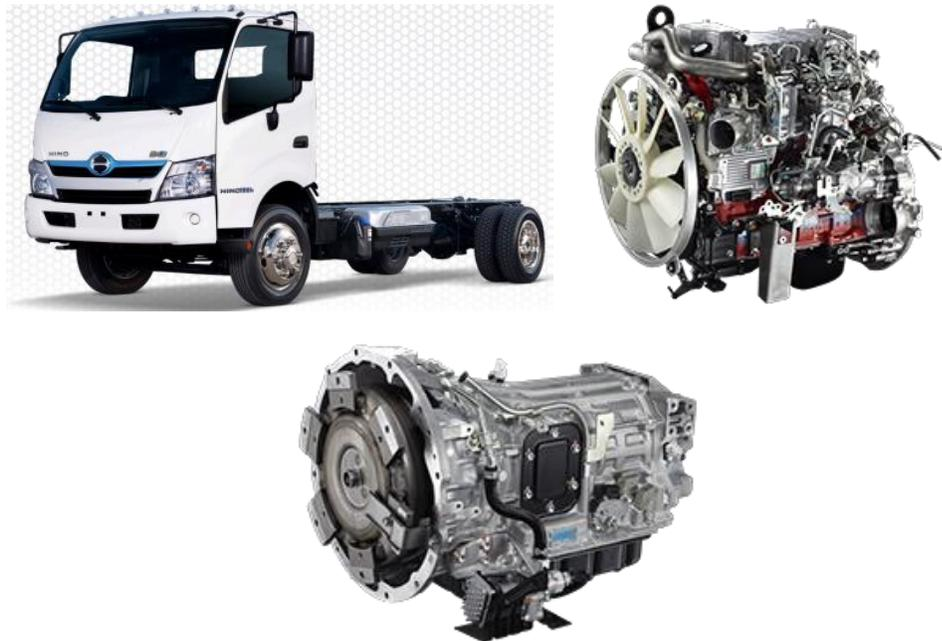
Figure 20: HINO 195h diesel-electric hybrid system (images from HINO Trucks)
