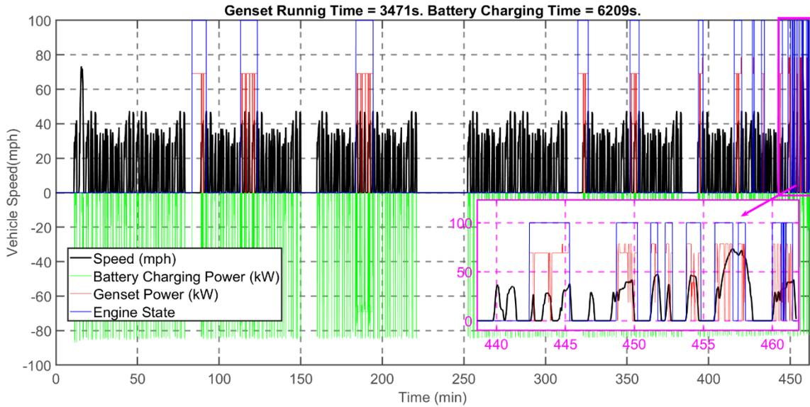
Figure 64: Genset power, engine state, battery power for the speed profile
