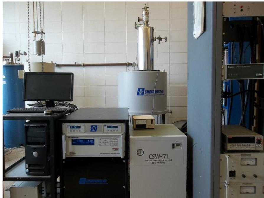
Figure 62. The 12 T conduction-cooled superconducting magnet system used to measure the magnetic properties of the superconducting cables. The central gray cylinder is the cryogen-free magnet with a room temperature bore.
