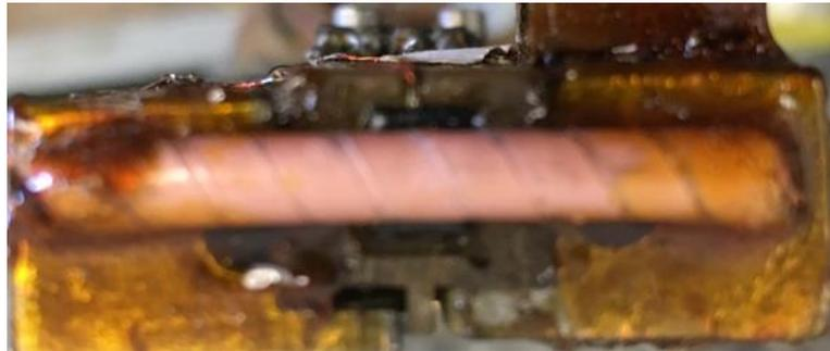
Figure 64. A CORC<sup>®</sup> cable section mounted onto the end of the sample holder. GE varnish is used to adhere the ends of the sample to the holder.
