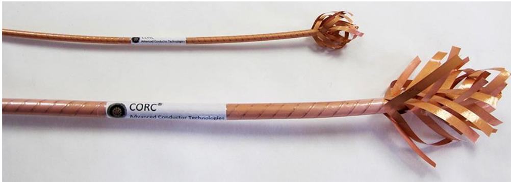
Figure 61. A CORC<sup>®</sup> wire (top of figure) and CORC<sup>®</sup> cable (bottom of figure), from [99].
