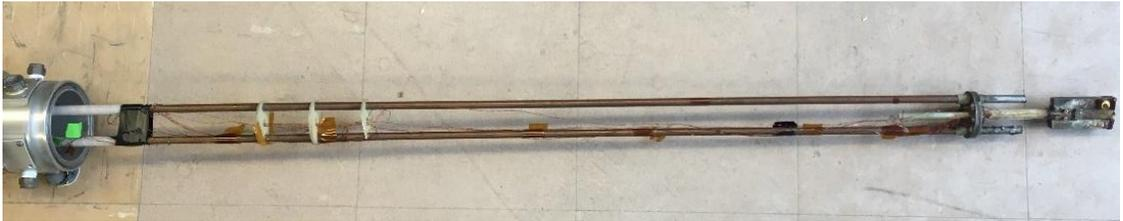
Figure 63. The sample holder used to mount the cable samples.
