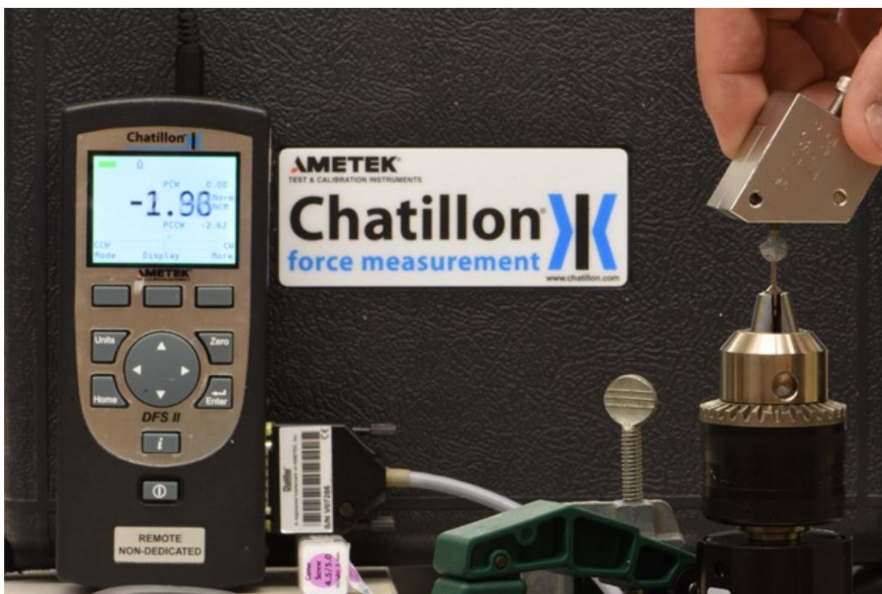
Figure 5. Measurement of peak counter-clockwise torque value (ie. removal or reversal torque).
